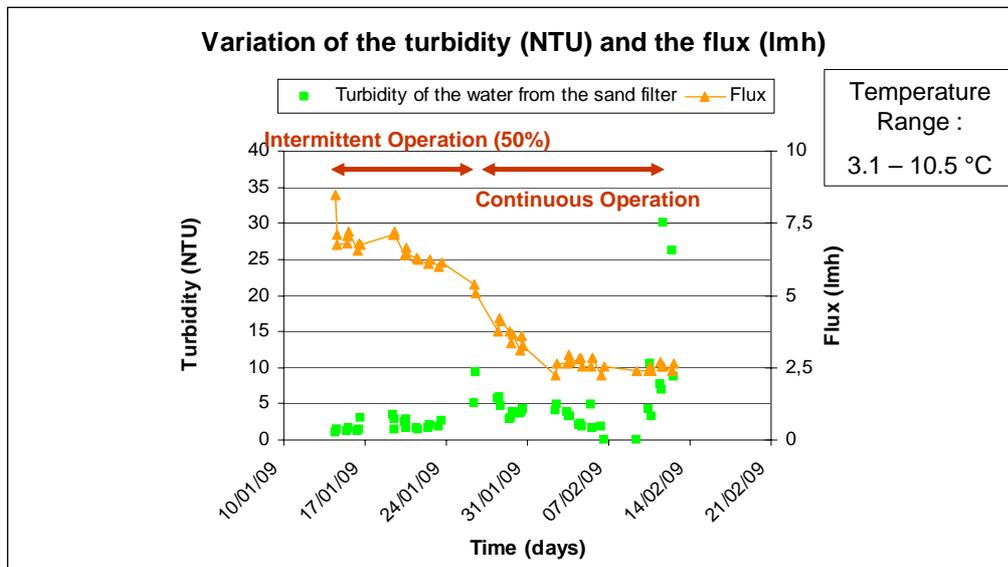
Figure 6 - Flux variation in regards to intermittent operation and turbidity feed
