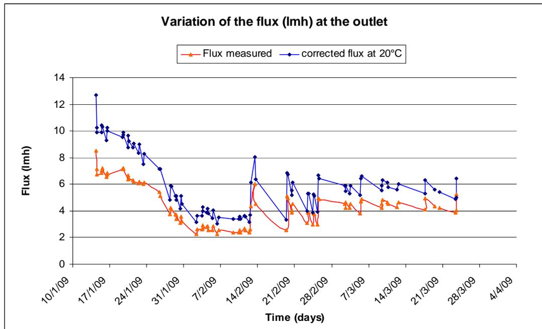
Figure 9 - Flux enhancement with a 20°C-correction
