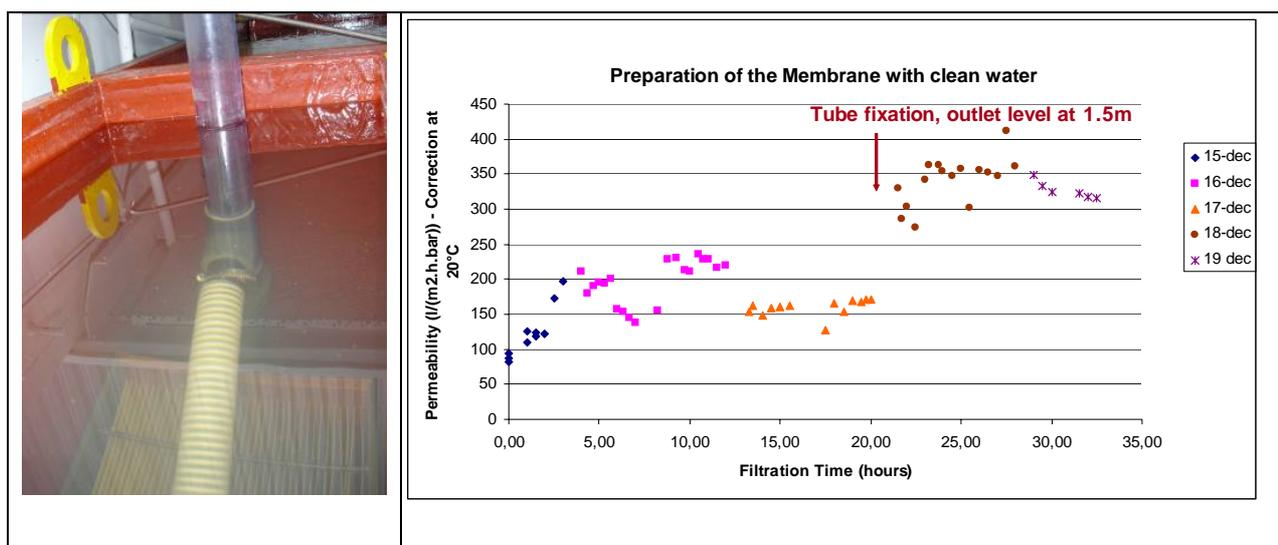
Figure 2 - Permeability Tests with the membrane before and after the addition of an open-air tube on the permeate pipe
