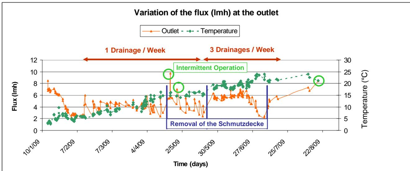
Figure 11 - Variation of the flux in function of the Operation and Maintenance conditions
