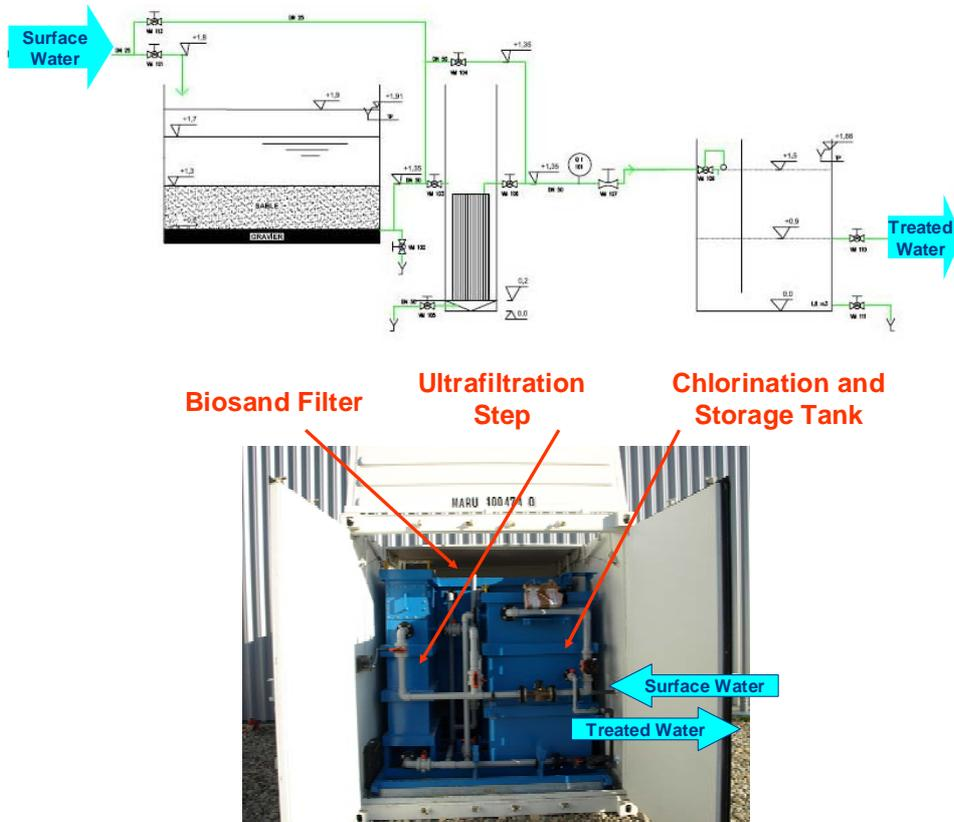
Figure 1 - Process Instrument Diagram and Photo of the compact unit
