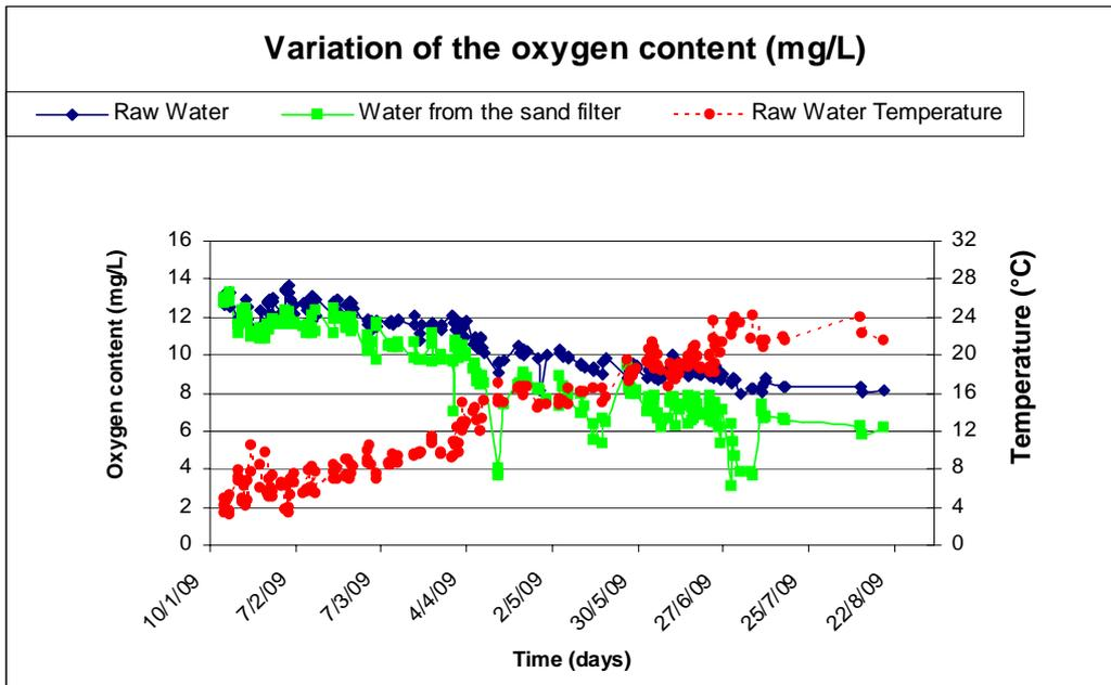
Figure 10 - Effect of temperature on the oxygen content
