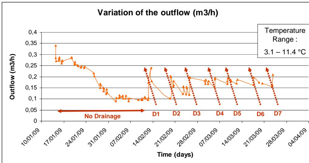
Figure 7 - Flux variation in regards to the drainage frequency
