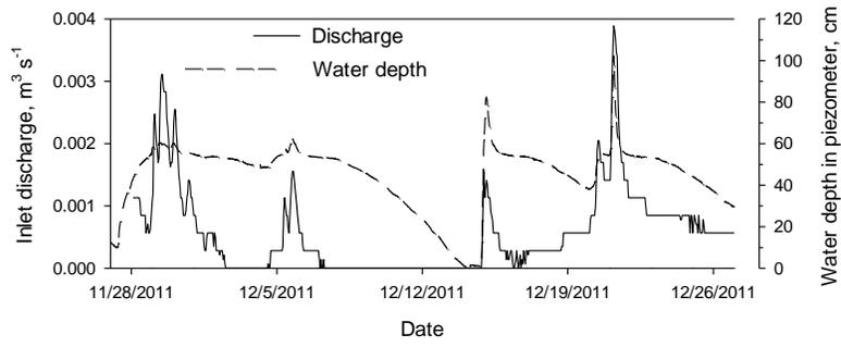
Fig. 6. Temporal variation in inlet discharge and water depth during the November-December 2011 event. Water depth was measured in the T3 piezometer.
