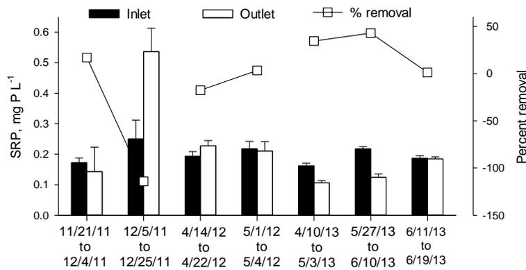
Fig. 12. Percent removal of soluble reactive P (SRP) during the course of the study. Negative values indicate a net release of SRP from the bioswale. Bars represent standard errors.
