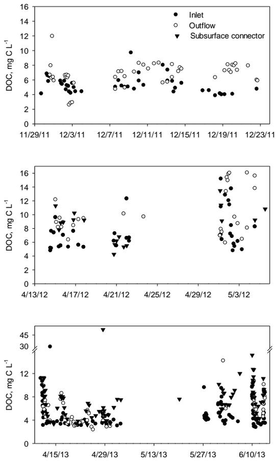
Fig. 13. Dissolved organic carbon (DOC) concentration at the inlet, T3 piezometer and outflow of the bioswale during wet events in autumn 2011 (top), spring 2012 (middle) and spring 2013 (bottom). Note the scale difference for DOC and ORP during the spring 2013 event.
