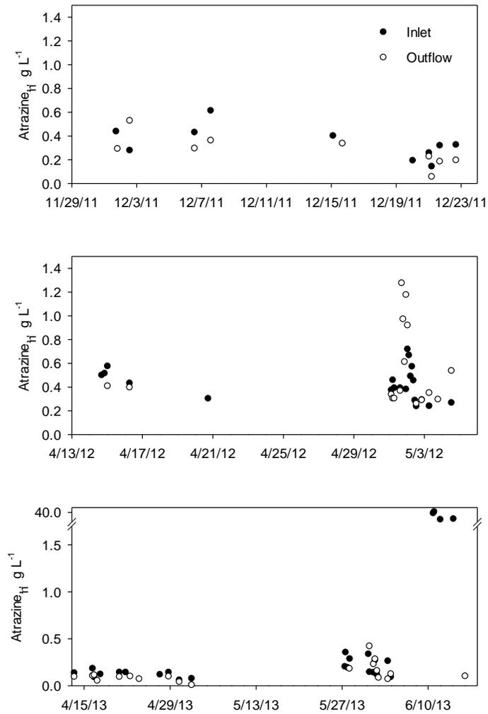
Fig. 17. Atrazine concentration in the inlet and outflow of the bioswale during wet events in autumn 2011 (top left), spring 2012 (middle left) and spring 2013 (bottom left). Atrazine concentration in the inlet and subsurface connector (top right). Note the spring 2013 event does not include the data for June 6 to June 19 due to large differences in atrazine concentration between the April and early June samples. The June 6-19 data is listed in Table 3.
