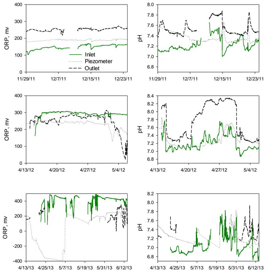
Fig. 14: Oxidation-reduction potential (ORP) (left) and pH (right) in the inlet, T3 piezometer and outflow of the bioswale during wet events in autumn 2011 (top), spring 2012 (middle) and spring 2013 (bottom).
