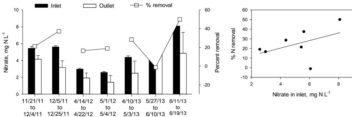
Fig. 9. Percent removal of nitrate during the course of the study (left), and relationship between NO<sub>3</sub><sup>-</sup> concentration in the inlet and % N removal. Bars represent standard errors.
