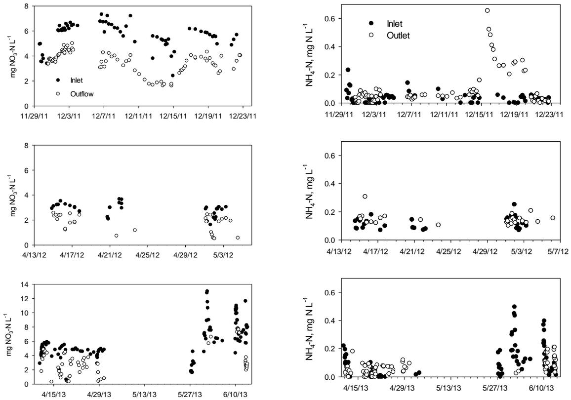
Fig. 7. Nitrate (left panel) and ammonium (right panel) concentration in the inlet and outflow of the bioswale during wet events in autumn 2011 (top), spring 2012 (middle) and spring 2013 (bottom). Note the scale difference for the spring 2013 event.
