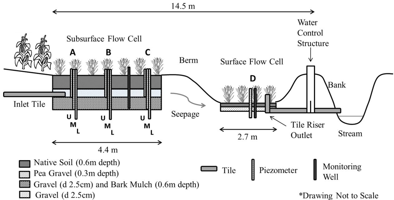
Fig. 2. Cross-sectional view of bioswale showing subsurface flow and surface flow cells, along with the approximate location of piezometers and monitoring wells.
