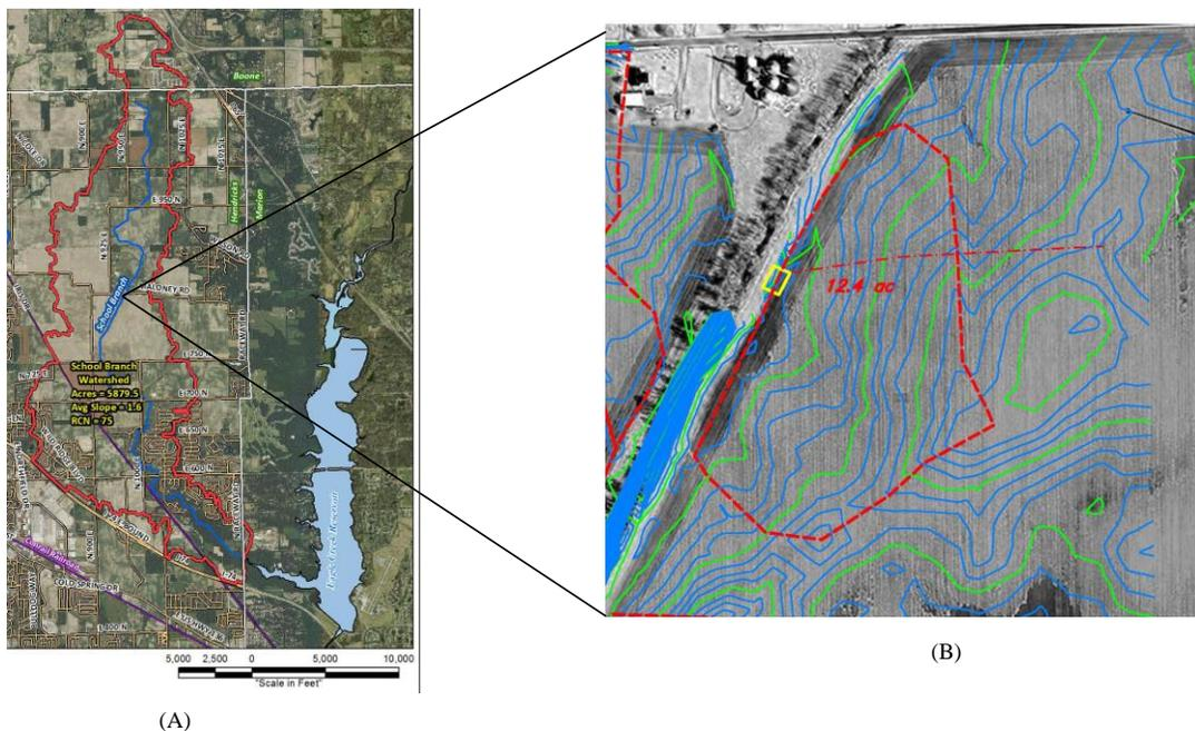
Fig. 1. Location of the bioswale in the School Branch watershed (A). The potential surface drainage area of the bioswale is shown in insert B. The straight red line depicts the subsurface tile drain intercepted by the bioswale (yellow box).
