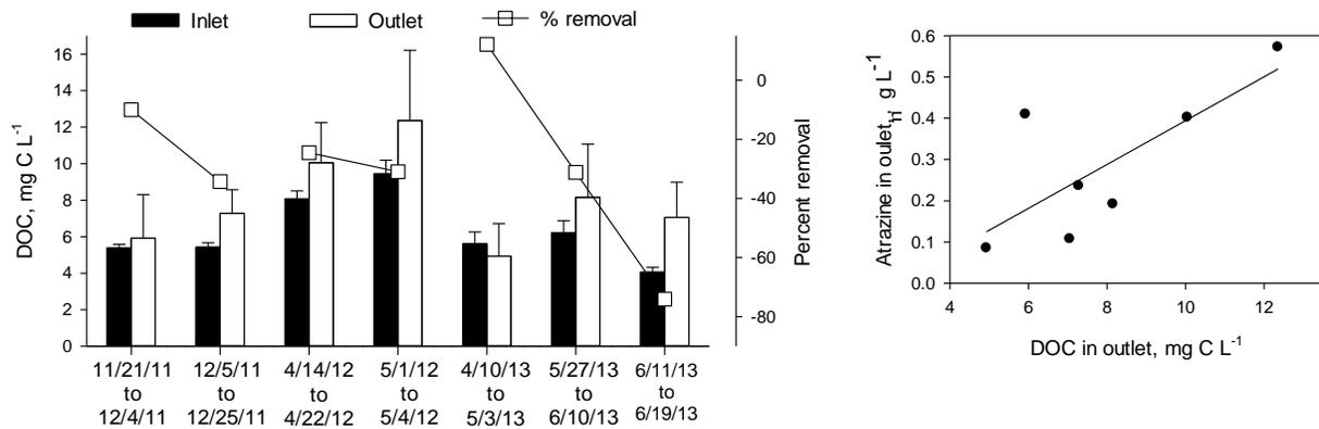
Fig. 16. Dissolved organic C (DOC) balance of the bioswale during the course of the study (left), and relationship between average atrazine and DOC concentration in the outlet (right). Positive values correspond to net gain while negative values indicate a net loss of C from the system. Bars represent standard errors.
