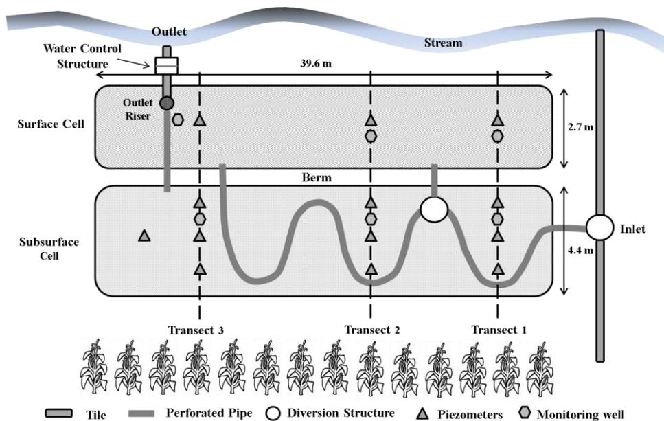
Fig. 3. Top-down view of water flow direction through the various compartments of the bioswale.
