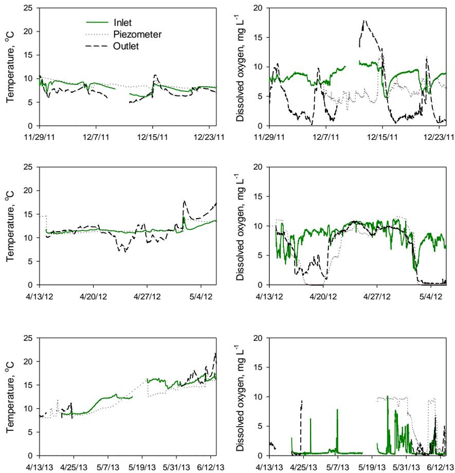
Fig. 10: Water temperature and dissolved oxygen at the inlet, T3 piezometer and outflow of the bioswale during wet events in autumn 2011 (top), spring 2012 (middle) and spring 2013 (bottom).
