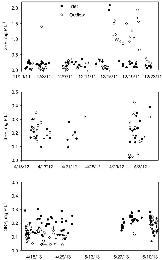
Fig. 11. Concentration of soluble reactive P (SRP) in the inlet and outflow of the bioswale during wet events in autumn 2011 (top), spring 2012 (middle) and spring 2013 (bottom). Note the scale difference for the autumn 2011 event.
