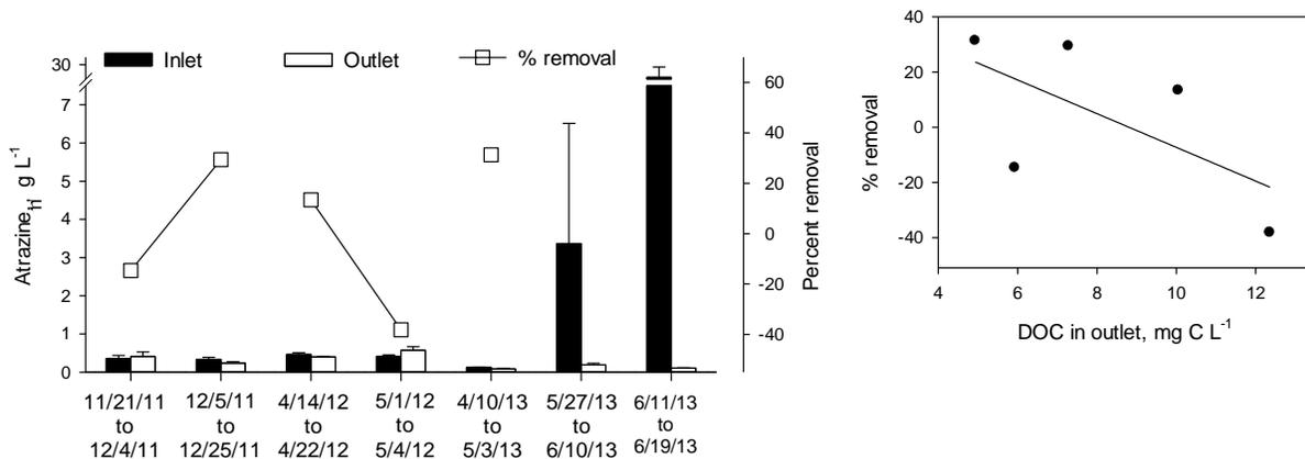
Fig. 18. Percent removal of atrazine in the bioswale during the course of the study (left), and relationship between atrazine removal rate during a period and average concentration of DOC in the outlet (right). Negative values indicate net release of atrazine from the bioswale. Bars represent standard errors.
