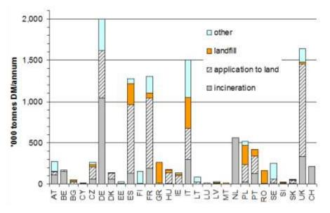
Figure 4: Sewage sludge valorisation and disposal routes in E27 + CH in 2010 (Milieu Ltd., 2010).
