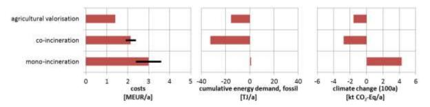
Figure 7: costs, fossil cumulative energy demand and climate change (100a) for different sludge disposal routes for a 1 million p.e. waste water treatment plant (P-REX reference system)
