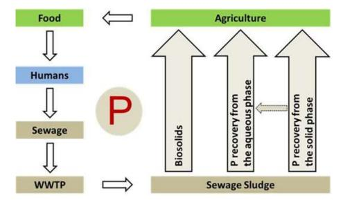
**Figure 3:** The three principal routes for P recovery and recycling from the wastewater stream as a nutrient. Wastewater REUSE for irrigation is not included. (Kabbe, 2013).
