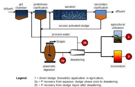
Figure 5: Hotspots for P recovery from the wastewater stream (in centralised sanitation systems), (Kabbe, 2013).
