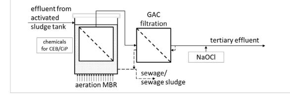
Figure 5 Basic flow sheet for aerated MBR, GAC filtration for colour removal and chlorination
