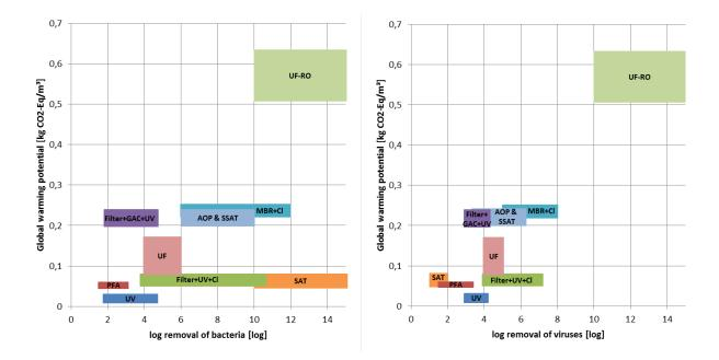
Figure 10 Range in global warming and risk reduction potential for selected treatment trains Llog removal of bacteria (left) and viruses(right) for selected treatment trains. Assumed travel time for SAT: 100-200 d and for SSAT: 30-35 d.
