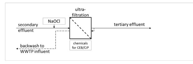
Figure 8 Basic flow sheet for ultrafiltration (UF)
