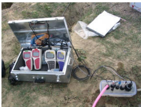
**Figure 4.14** Measuring in-situ parameters on site (flow-through cell, measuring devices in steel box).
