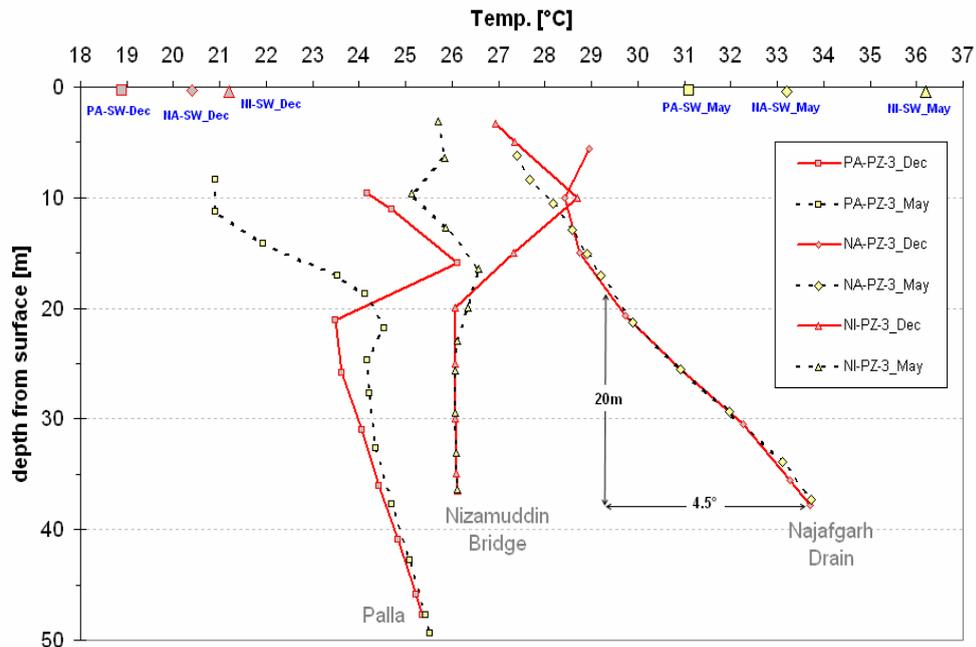
**Figure 4.18** Temperature logs from the months of December 2006 and May 2007, showing actual temperature gradient in the deepest piezometers of each field site. Surface water temperatures of adjacent water bodies and temperature gradient at Najafgarh Drain are also indicated.
