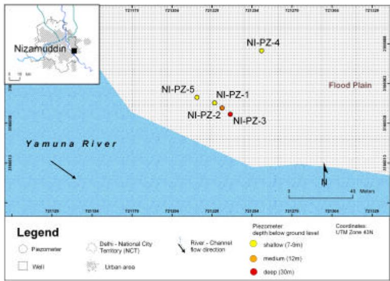
Figure 4.12 Piezometer setup at Nizamuddin bridge.
