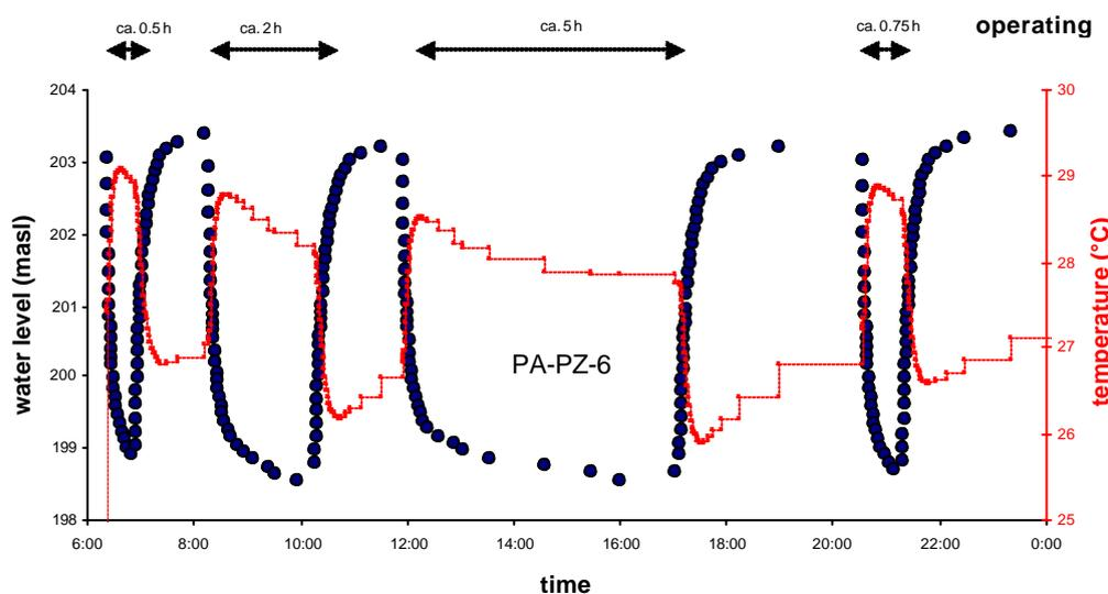
Figure 4.15 Hydraulic heads and temperature log for the Palla well. Recorded at observation well (PA-PZ-6).
