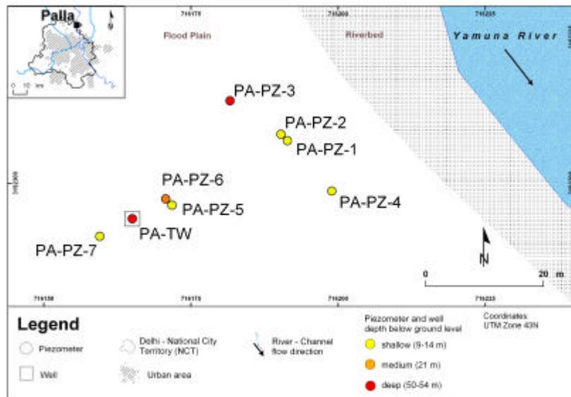
Figure 4.8 Piezometer setup in Palla.
