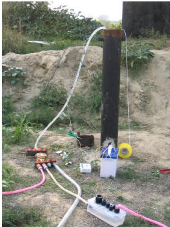
Figure 4.13 Measuring setup at a piezometer (flow-through cell, accumulator, light plummet, water meter)
