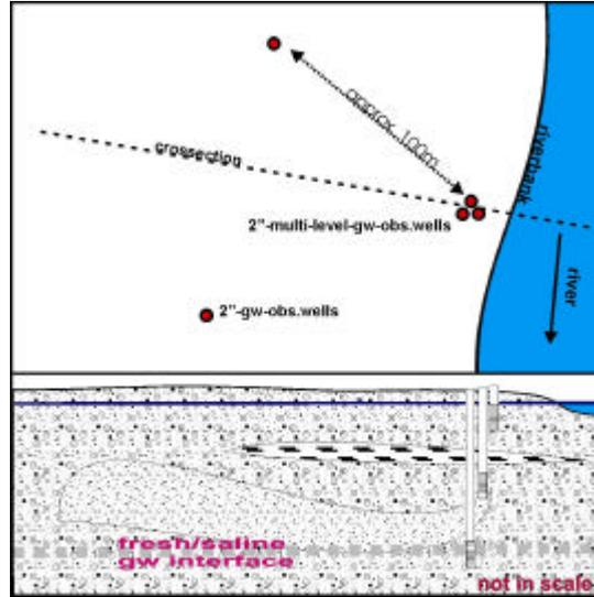
Figure 4.5 General piezometer setup.
