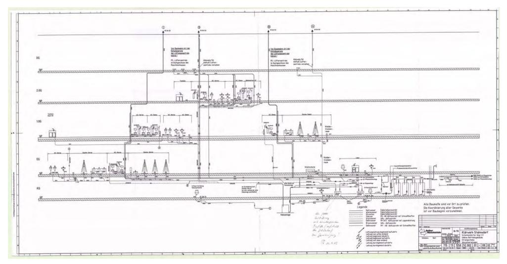
Line scheme of the sanitation system inside the office building
