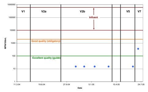
Fig. 3.5.6.8: Faecal coliforms in the influent and effluent of the constructed wetland
