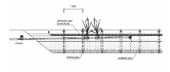
Fig. 2.4.16: Constructed wetland, cross section
