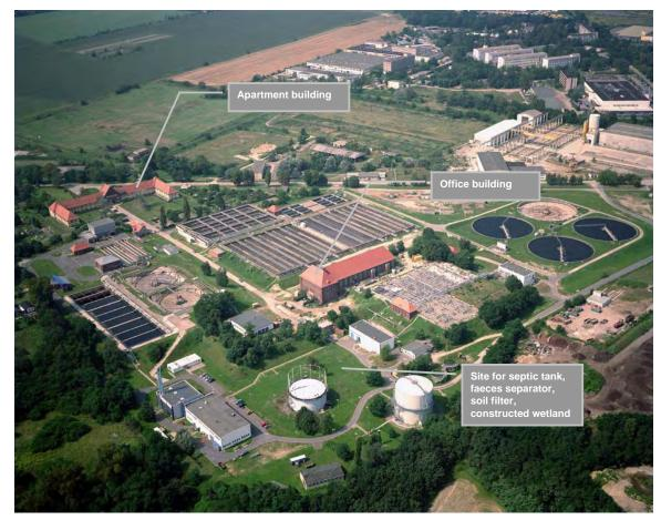
Fig. 2.1.1: Aerial view of WWTP Stahnsdorf and SCST-project site
