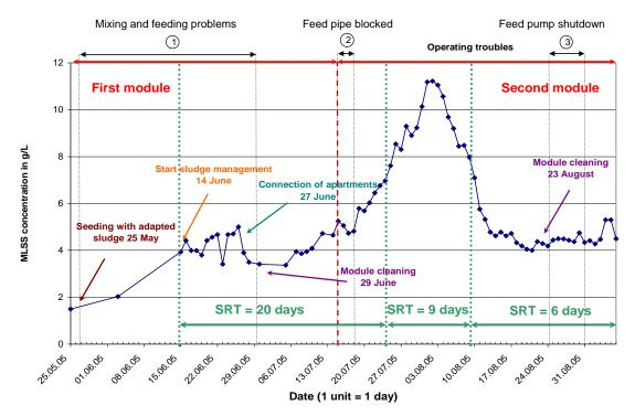
Fig. 3.5.7.1: MLSS evolution in the reactor and operational conditions
