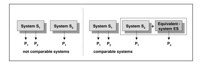
Figure 3: Principle of system expansion
