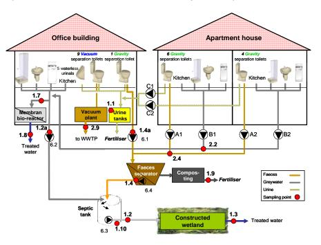
**Fig. 2.3.7:** Flow scheme of *Variant V7* (without soil filter, but treatment of faecal filtrate, operation of membrane bio-reactor including greywater from apartment house)
