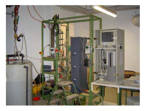
Fig. 2.4.6: Membrane bio-reactor
