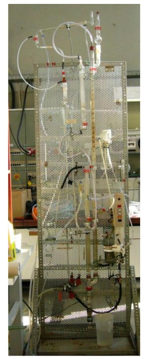
Picture 6: Steam stripping unit in laboratory scale
