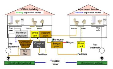
**Fig. 6.1:** New sanitation concepts with *gravity* separation toilets in the office building and with *vacuum* separation toilets in the apartment house of the WWTP Stahnsdorf
