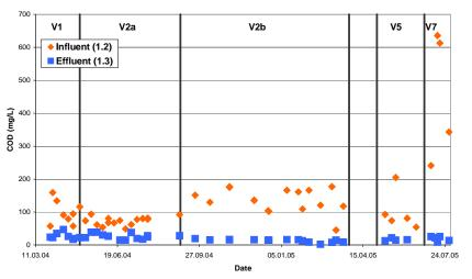
Fig. 3.5.6.3: COD of the influent and effluent of the constructed wetland (24 h composite sample)
