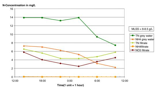
Fig. 3.5.7.2: Evolution of nitrogen concentration in grey water and filtrate during 24 hours
