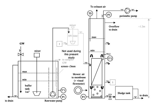
Fig. 2.4.8: Flow scheme of the membrane bio-reactor
