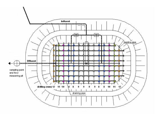
Fig. 2.4.17: Constructed wetland, distribution system
