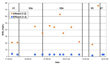
**Fig. 3.5.6.4**: BOD<sub>5</sub> of the influent and effluent of the constructed wetland (24 h composite sample)
