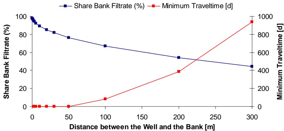
Figure 31 Influence of varying production well distances to the bank for a constant pumping rate of  $0.044 \text{ m}^3/\text{s}$
