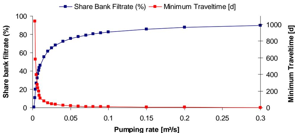
Figure 30 Influence of varying pumping rates on bank filtration share and minimum traveltime. The distance between the bank and the well is 63 meters. Note that below a pumping rate of  $0.002 \text{ m}^3/\text{s}$ , the minimum traveltime becomes infinite, since the hydraulic gradient between bank and well is too low
