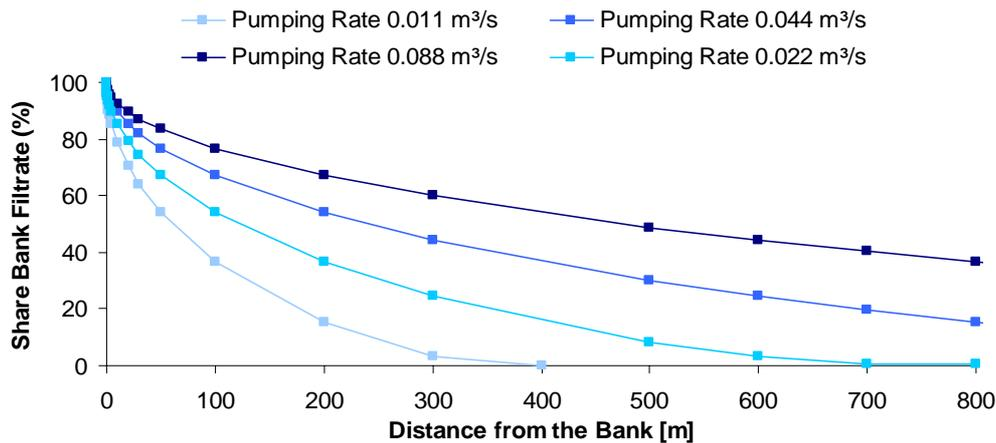
*Figure 33* Influence of varying pumping rates (coloured lines) and different well distances to the bank (squares) on the share of bank filtrate
