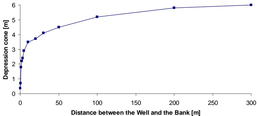
Figure 32 Influence of the distance between one well and the bank on the depression cone depth
