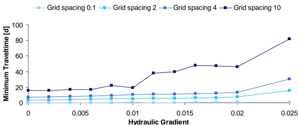
Figure 38 *Influence of the grid spacing on the minimum traveltime for a pumping well at 20m from the bank*
