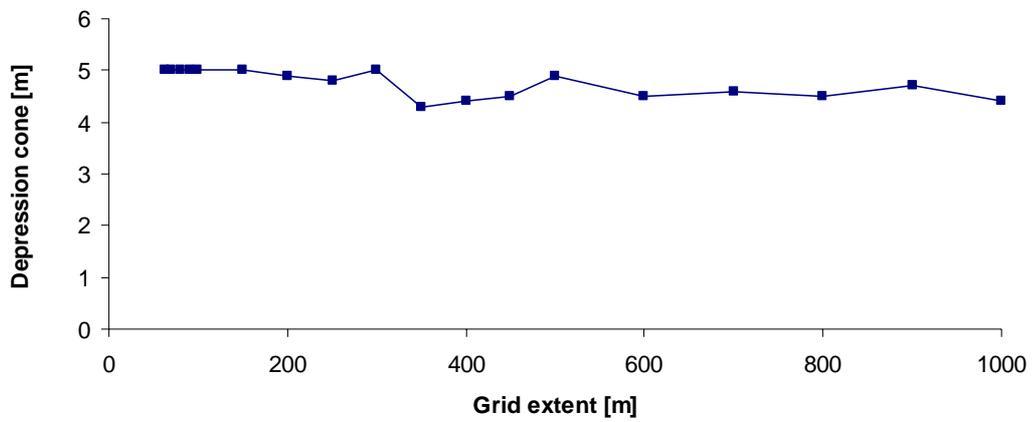
Figure 17 Influence of the grid extent on the depression cone calculation
