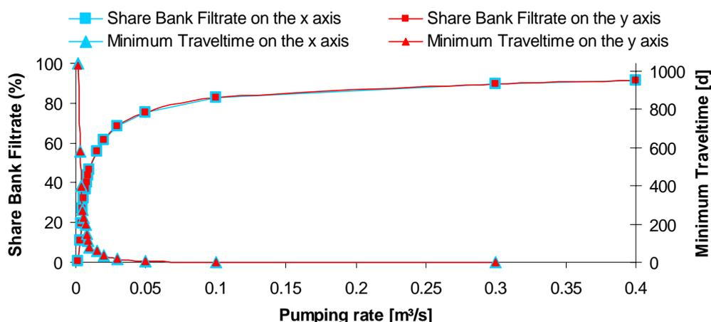
Figure 28 Influence of the orientation of the bank on the share bank filtrate and the minimum traveltime calculation
