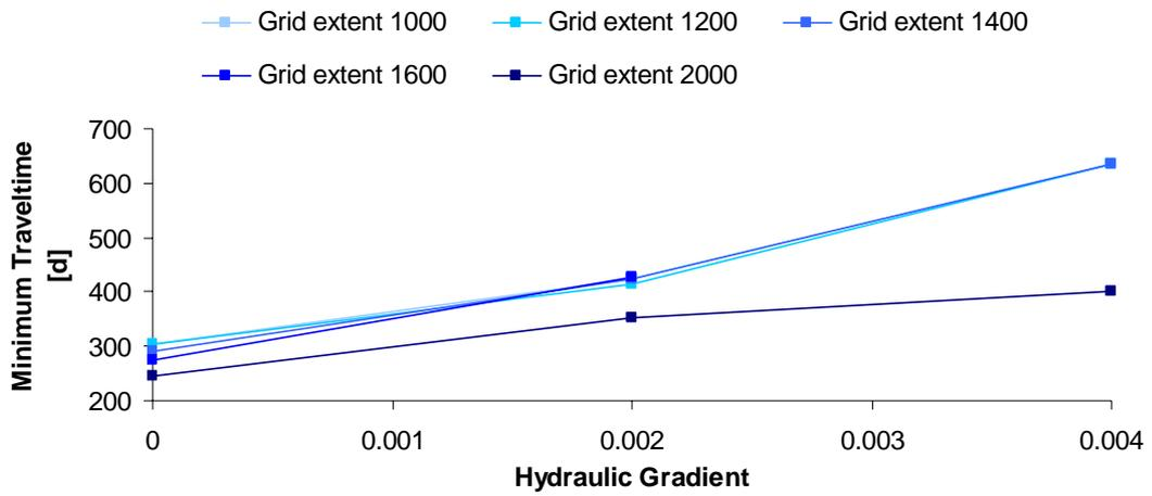
Figure 40 Influence of the grid extent on the minimum traveltime for a distance between the well and the bank of 200 m
