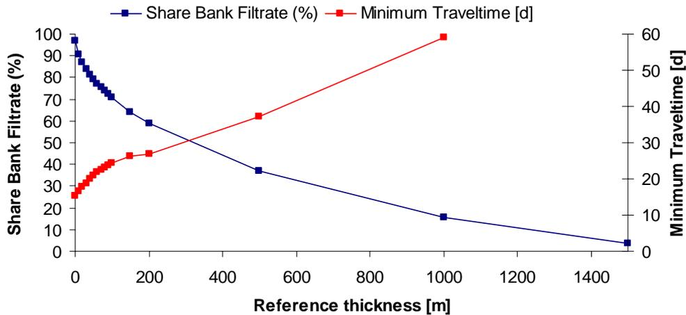
Figure 26 Influence of reference thickness on bank filtration share and minimum traveltime calculation
