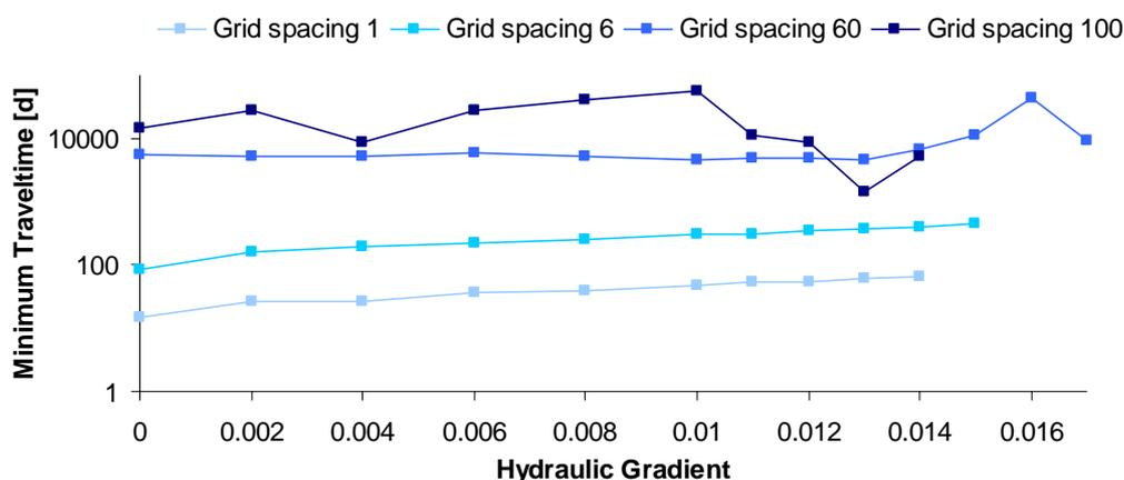
Figure 37 *Influence of the grid spacing on the minimum traveltime for a pumping well at 63m from the bank*
