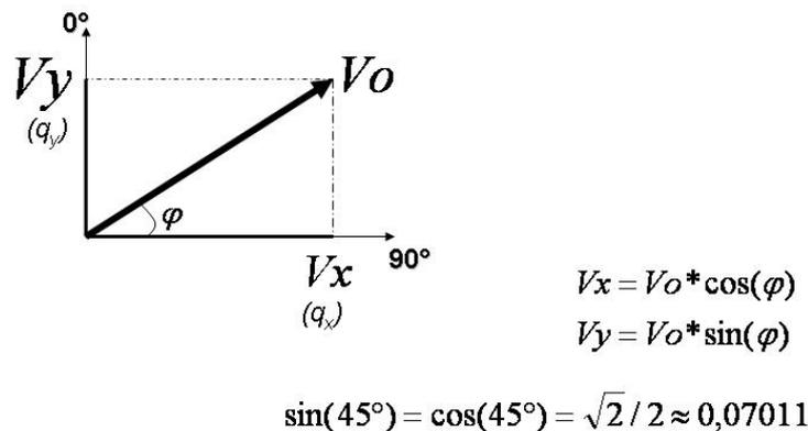
Figure 6 Baseflow ( $q_x$ ,  $q_y$ ) and velocity ( $V_x$ ,  $V_y$ ) vector components for an angle ( $\varphi$ ) of 45°
