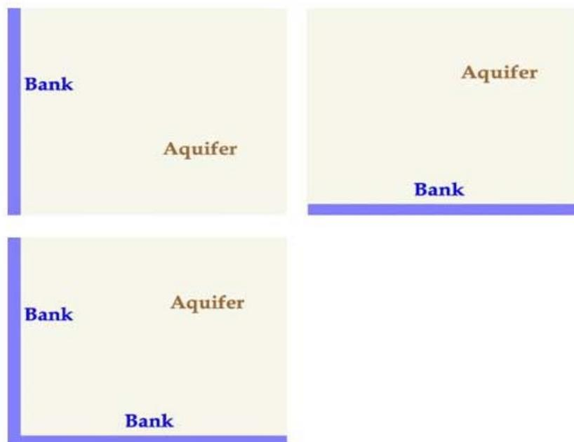
Figure 9 Bank orientation options: y-axis (upper left), x-axis (upper right) and both (lower left)
