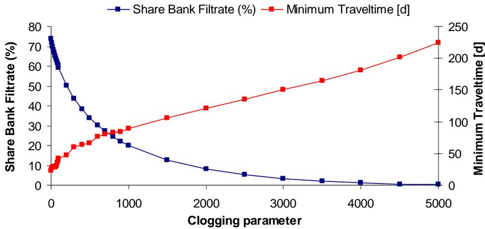
Figure 29 Influence of the clogging parameter on the share bank filtrate and the minimum traveltime
