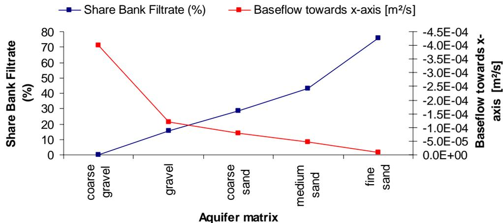
Figure 23 Influence of the hydraulic conductivity on the share bank filtrate (blue line) and baseflow (red line); no values are given for sandy silt and clay because the aquifer is partially running dry.
