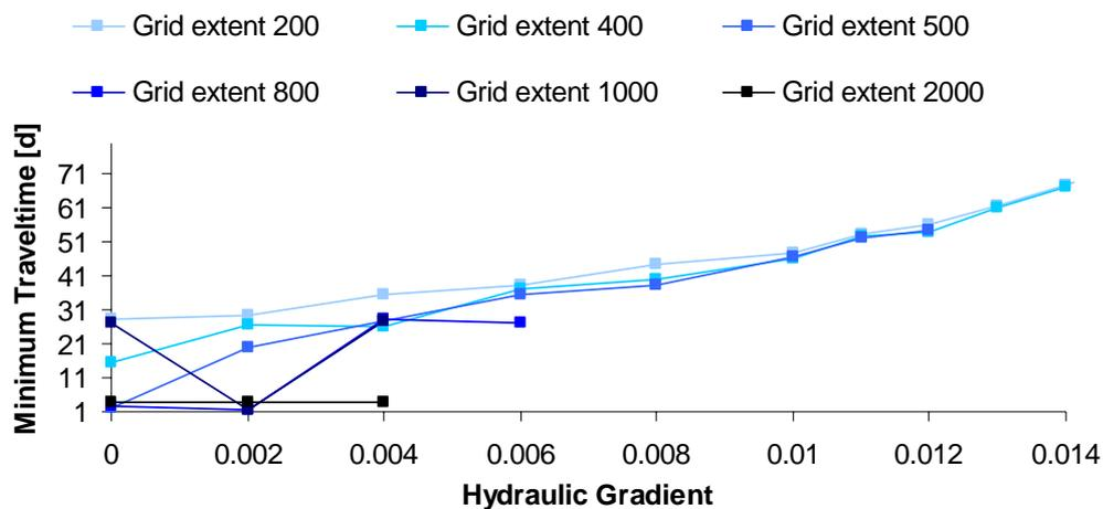
*Figure 39 Influence of the grid extent on the minimum traveltime for a distance between the well and the bank of 63 m*
