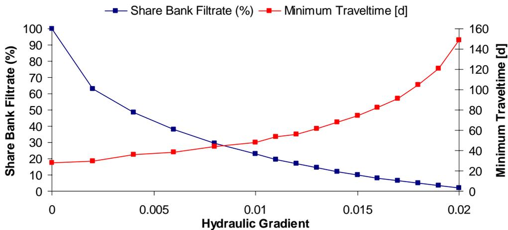
Figure 25 Influence of the hydraulic gradient on share bank filtrate and minimum traveltime. Grid parameters: [0:1:200] [-100:1:100]
