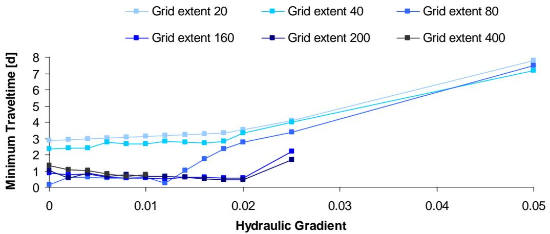
Figure 41 Influence of the grid extent on the minimum traveltime for a distance between the well and the bank of 20 m
