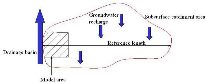
*Figure 7* Components of the hydrological balance: subsurface catchment area (red lines), groundwater recharge (small blue arrows) and reference length (black line). Note that the model area (black square with crossed lines) depends only on the user defined grid extent (Chapter 5.2) and has no influence on the baseflow calculation.
