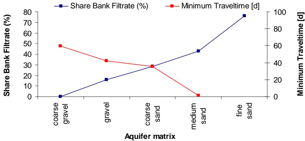
Figure 24 Influence of the hydraulic conductivity on the share bank filtrate (blue line) and the minimum traveltime (red line); no values are given for sandy silt and clay because aquifer is partially running dry.
