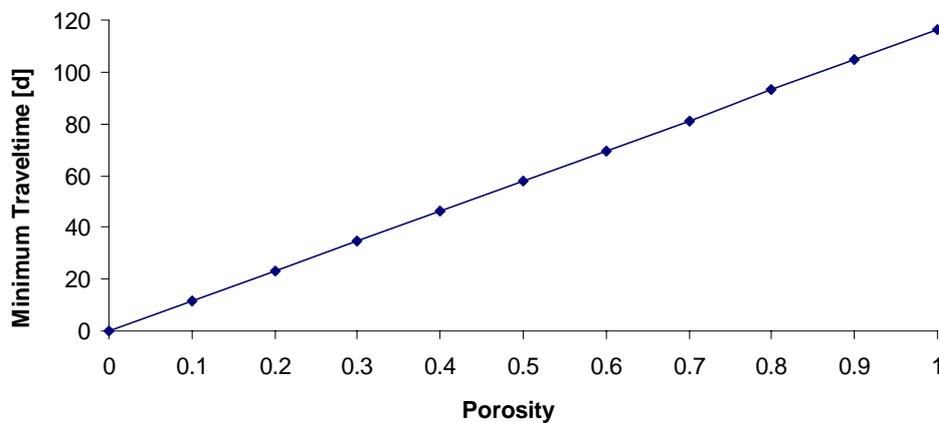
Figure 27 Influence of effective porosity on minimum traveltime calculation
