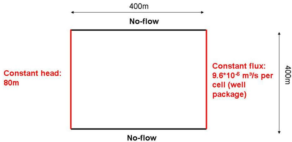
Figure 36 Boundary conditions for the site specific MODFLOW-2000 model;
