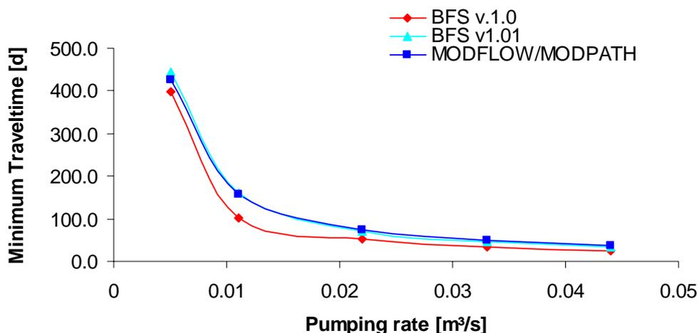
Figure 35 Accuracy of the minimum traveltime output for the two BFS versions (1.0 and 1.01) compared to the MODFLOW/MODPATH results for different pumping rates
