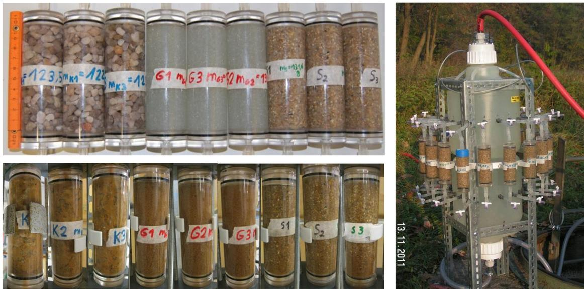
Figure 8: Mini columns before (top left) and after (bottom left) exposure and setup for installation at a drinking water production well (right) [SCHWARZMÜLLER et al. 2013]
