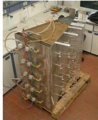
Figure 7: Model well tank design with measurement equipment.
