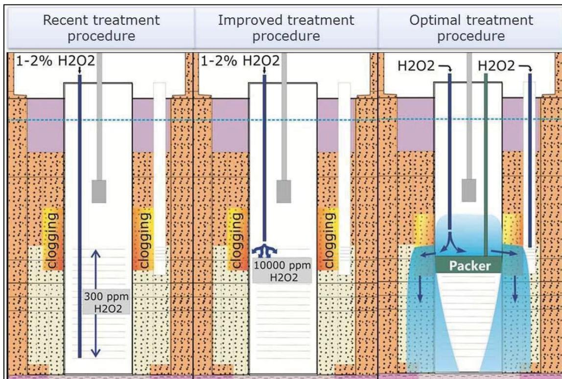
Figure 12: Comparison of old (left), and recommended improved (middle) and optimal (right) treatment application procedure
