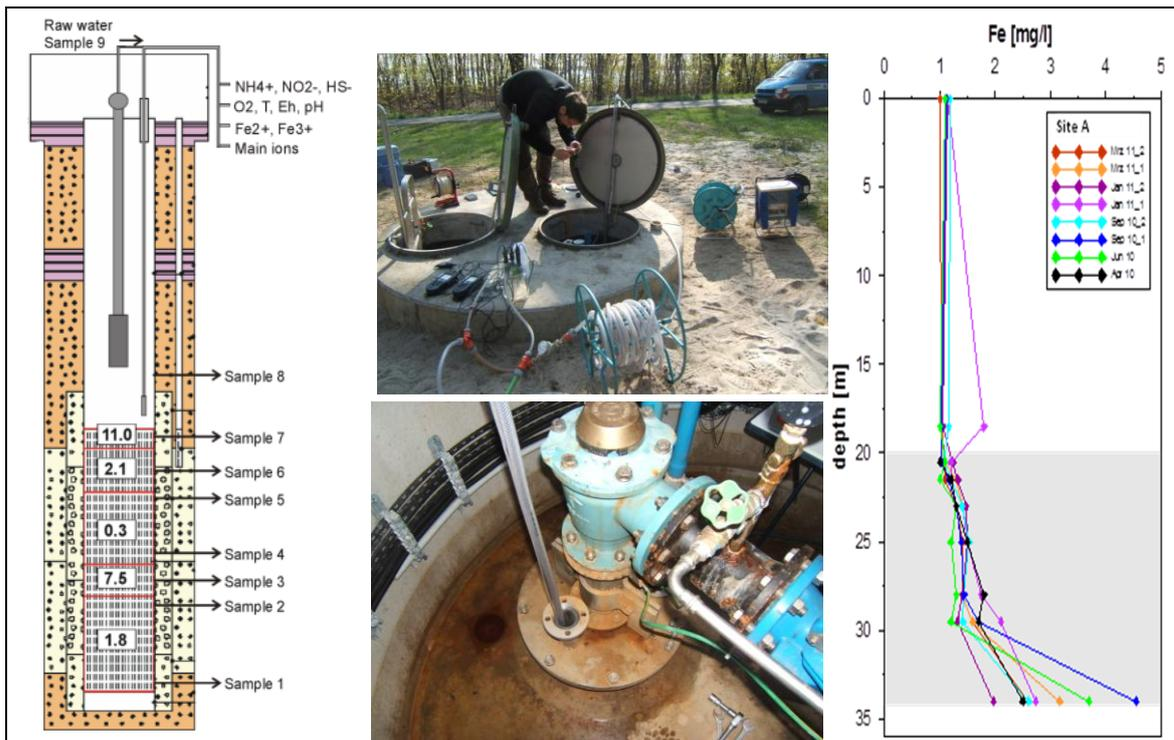
Figure 4: Scheme of depth-oriented sampling (left), procedure in the field (middle) and results interpretation (right). Sample depths correspond to the intake distribution indicated in the red boxes [MAIWALD et al. 2011]
