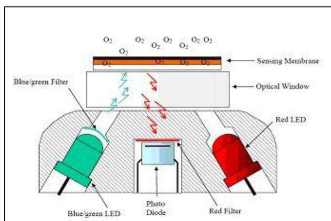
Figure 5: Principle of oxygen measurement with optodes [www.coastalwiki.org, accessed 06/2013]
