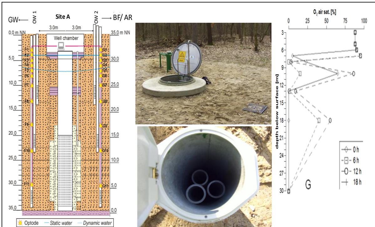
Figure 6: Transect design and location of optodes for in-situ oxygen measurements (left), field installations (middle) and results interpretation for one of the optode chains (right) [MAIWALD et al. 2011]
