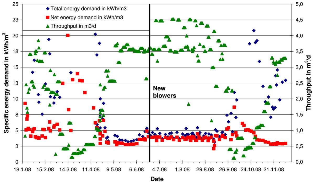
**Figure 68: Energy demand of the BUSSE prototype plant**
