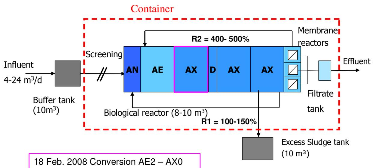
**Figure 28: Flow sheet of the MBR plant with process optimization**
