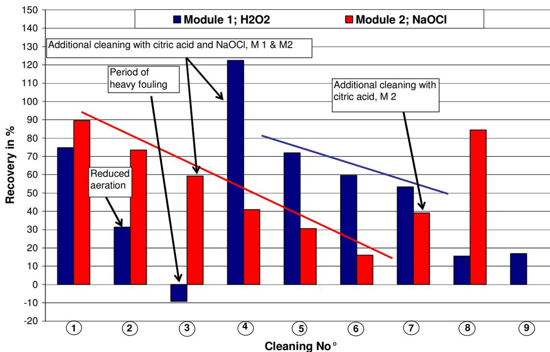
**Figure 41: Recovery of permeability after cleanings**
