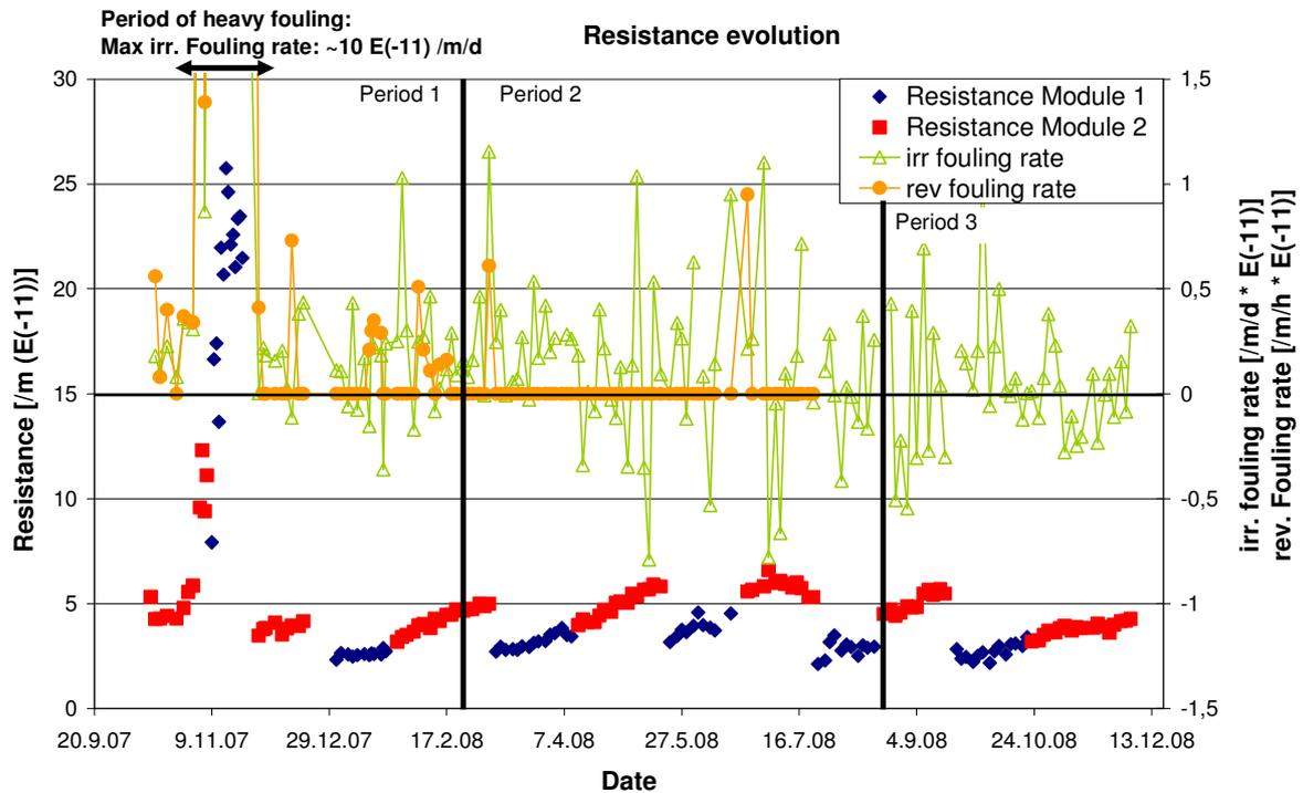
**Figure 48: Evolution of the filtration resistance, irr. and rev. fouling rate for the demonstration plant**
