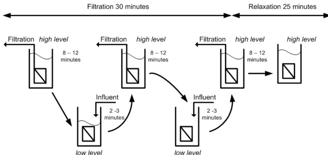
**Figure 58: Filtration cycle of prototype plant**
