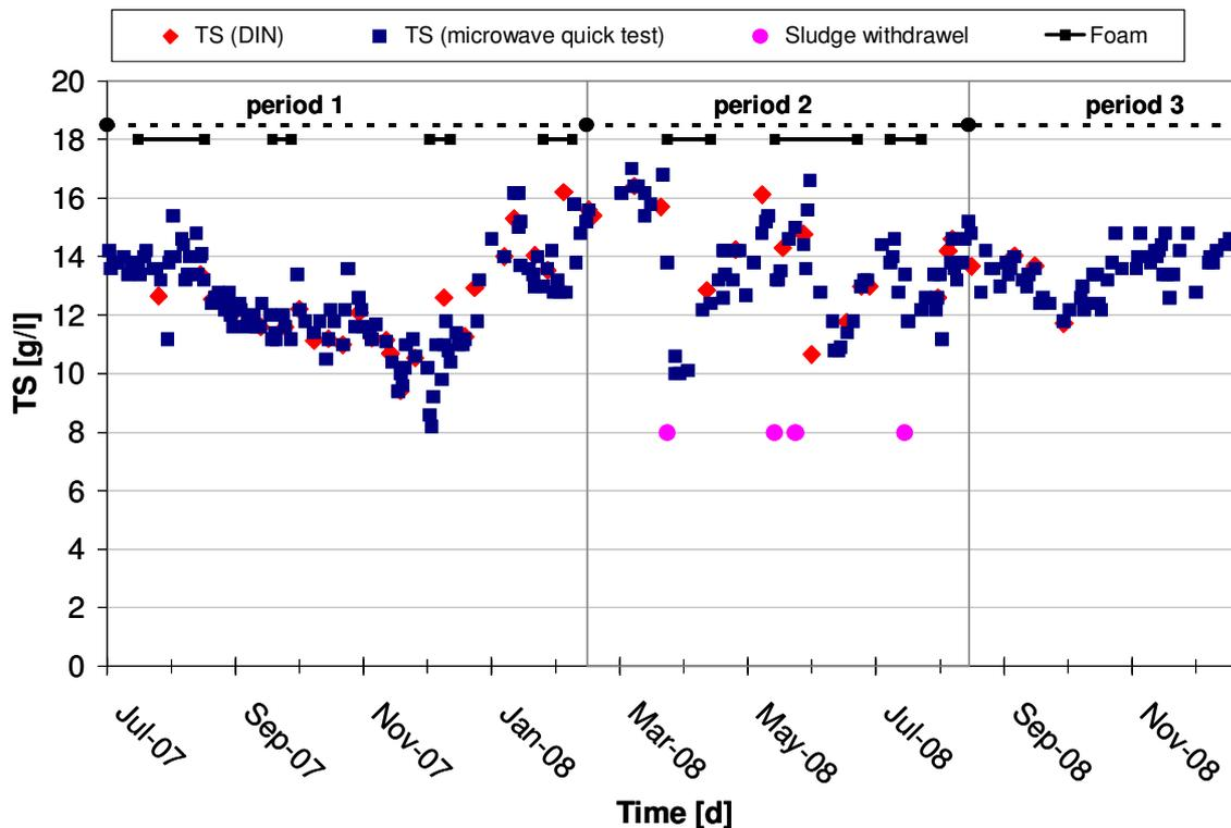
**Figure 13: Foam events and accidental sludge loss within the period of trials**
