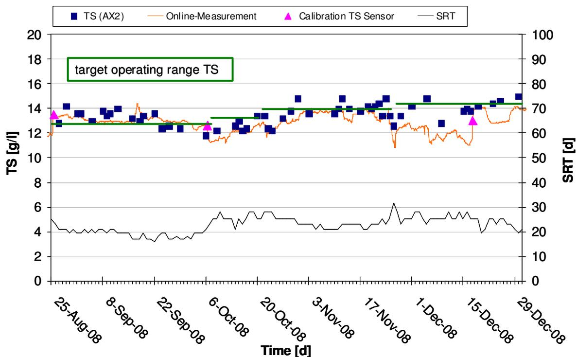
Figure 12: TS control: SRT adjustment relating to the TS online measurement
