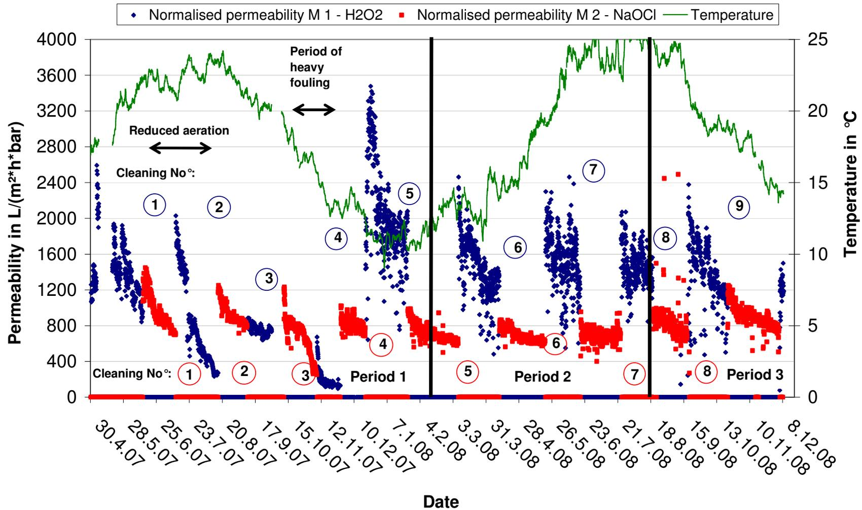
Figure 40: Permeability evolution indicating the cleaning events
