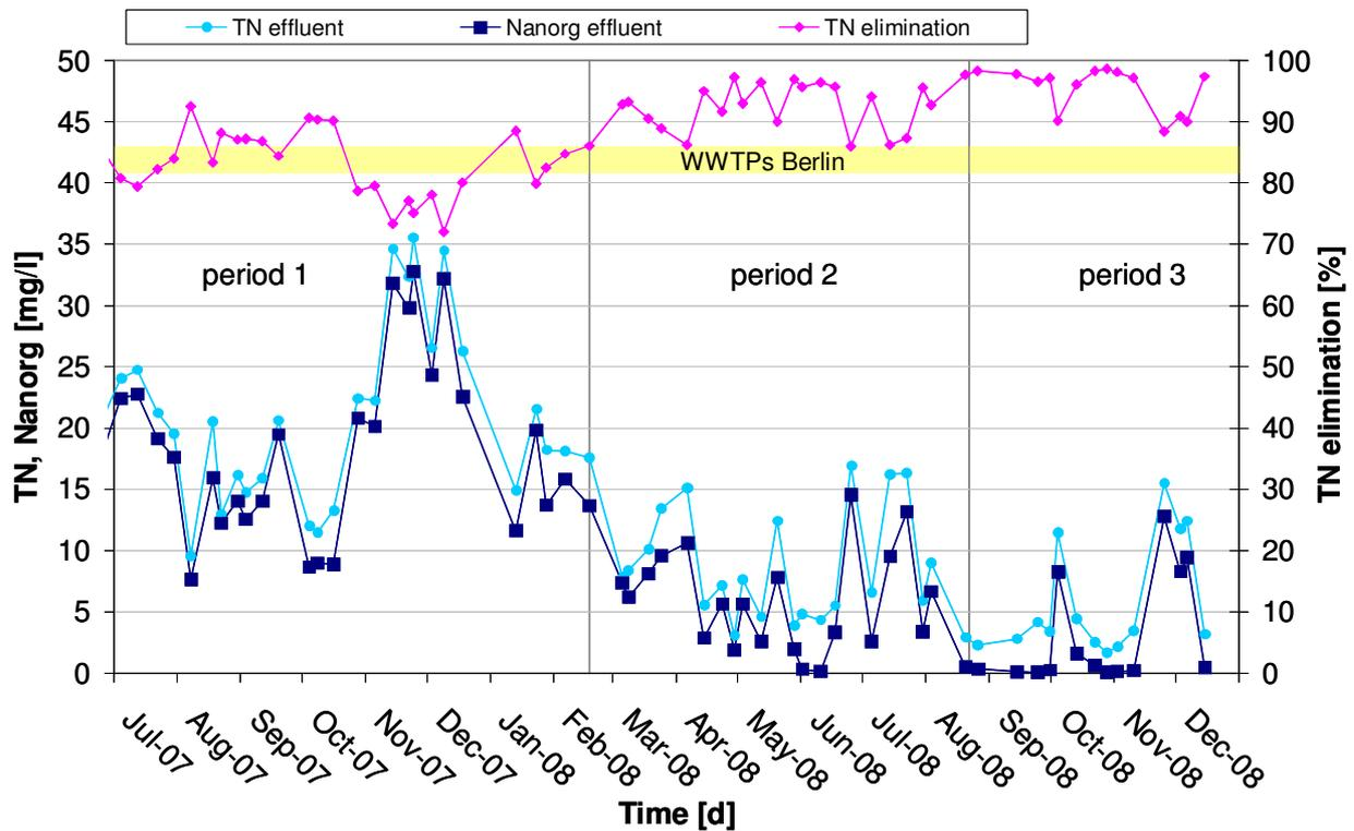
Figure 10 Total nitrogen and NO<sub>3</sub>-N effluent values and TN-elimination rate (24h samples)
