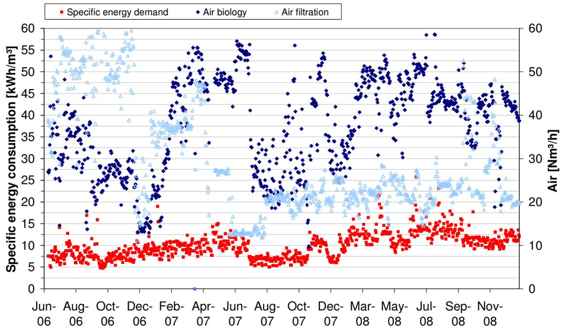
**Figure 21: Specific daily energy demand of the demonstration plant over time**
