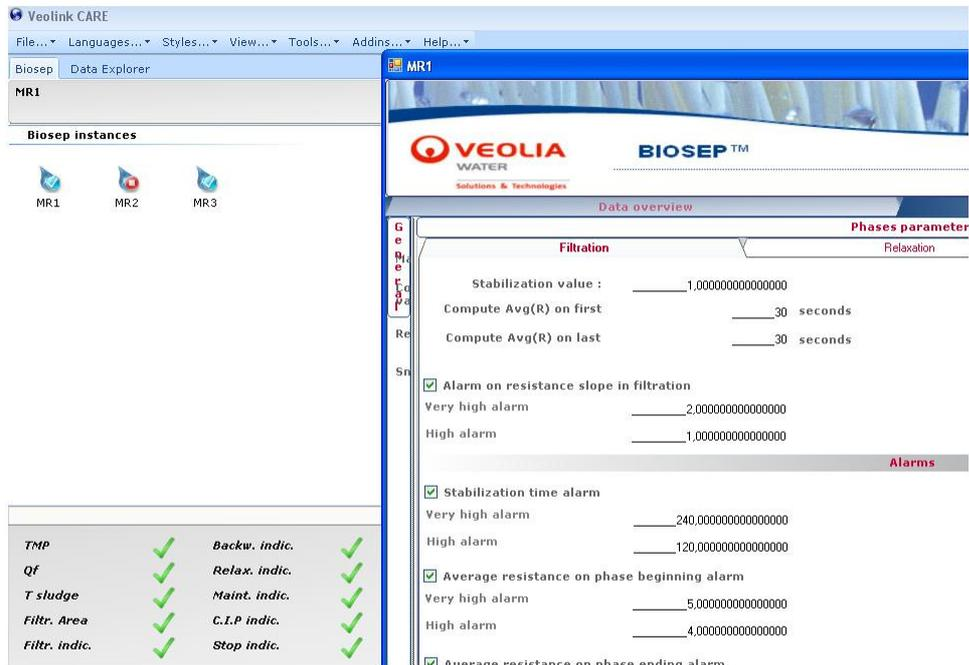
Figure 17: Filtration performance observation with alarm settings (Veolink®)
