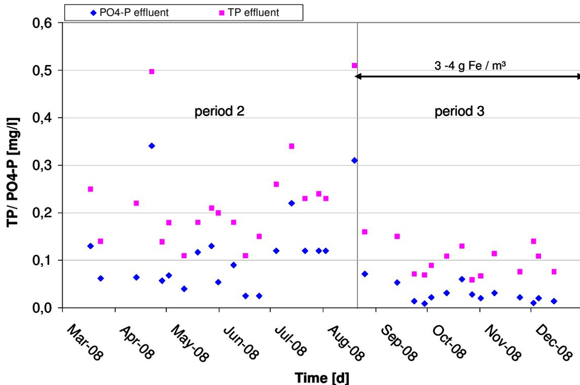
**Figure 35: Phosphorus effluent concentrations before and after precipitation (24 h samples)**
