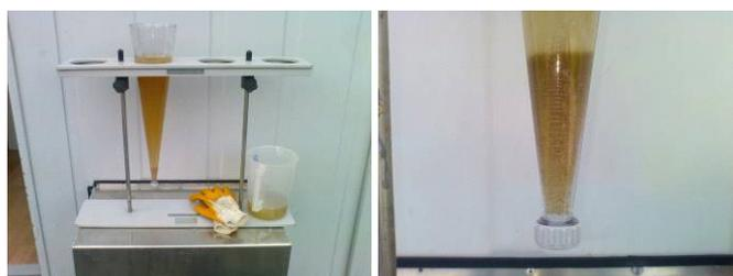
**Picture 2: Trials of sedimentation volume in Imhoff cone**
