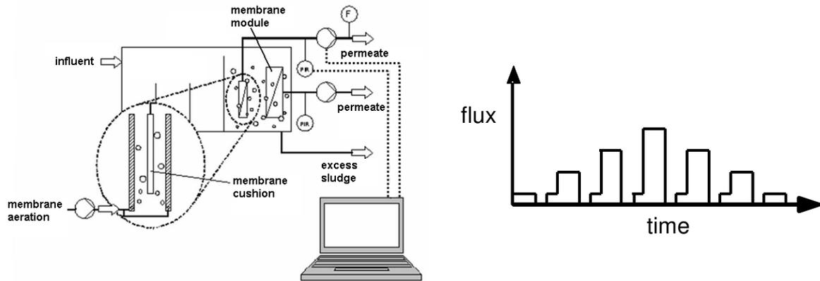
**Figure 42: Scheme of the *in situ* BFM test cell and  $J_c$  pre-step protocol**
