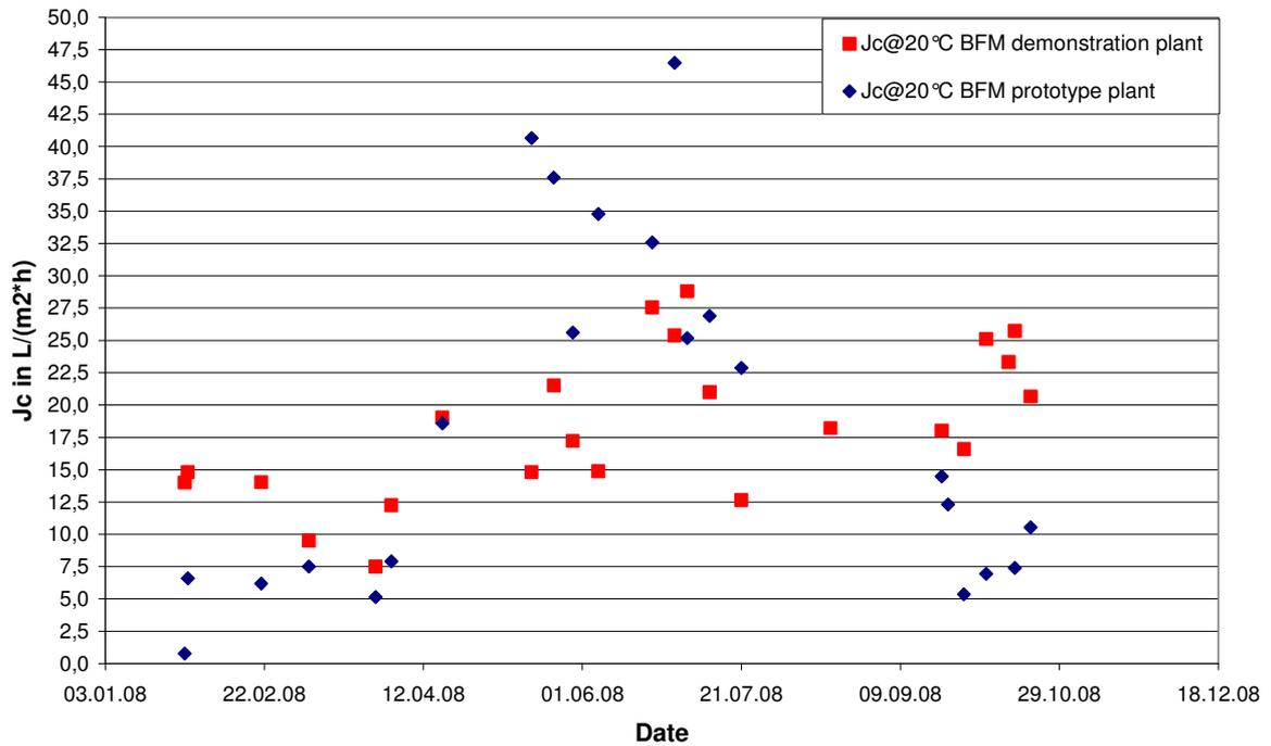
**Figure 44: Jc@20°C obtained with the BFM for both plants**
