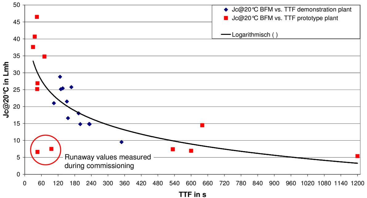
Figure 51: Critical flux in relation to TTF for both plants
