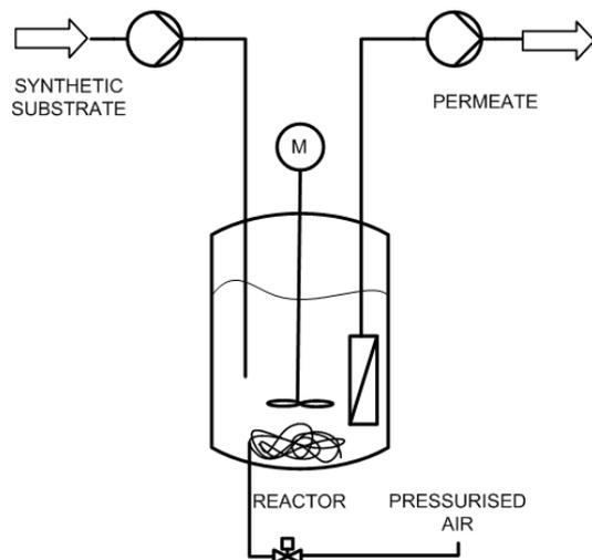
**Figure 31: Laboratory scale plant**
