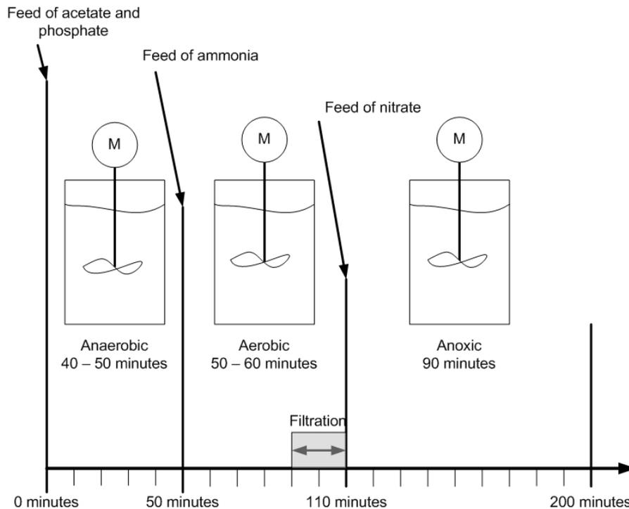
**Figure 32: Operation cycle with the biological conditions and times of dosage**
