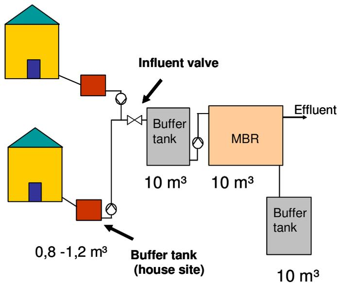
**Figure 2: Flow scheme of network and MBR plant**
