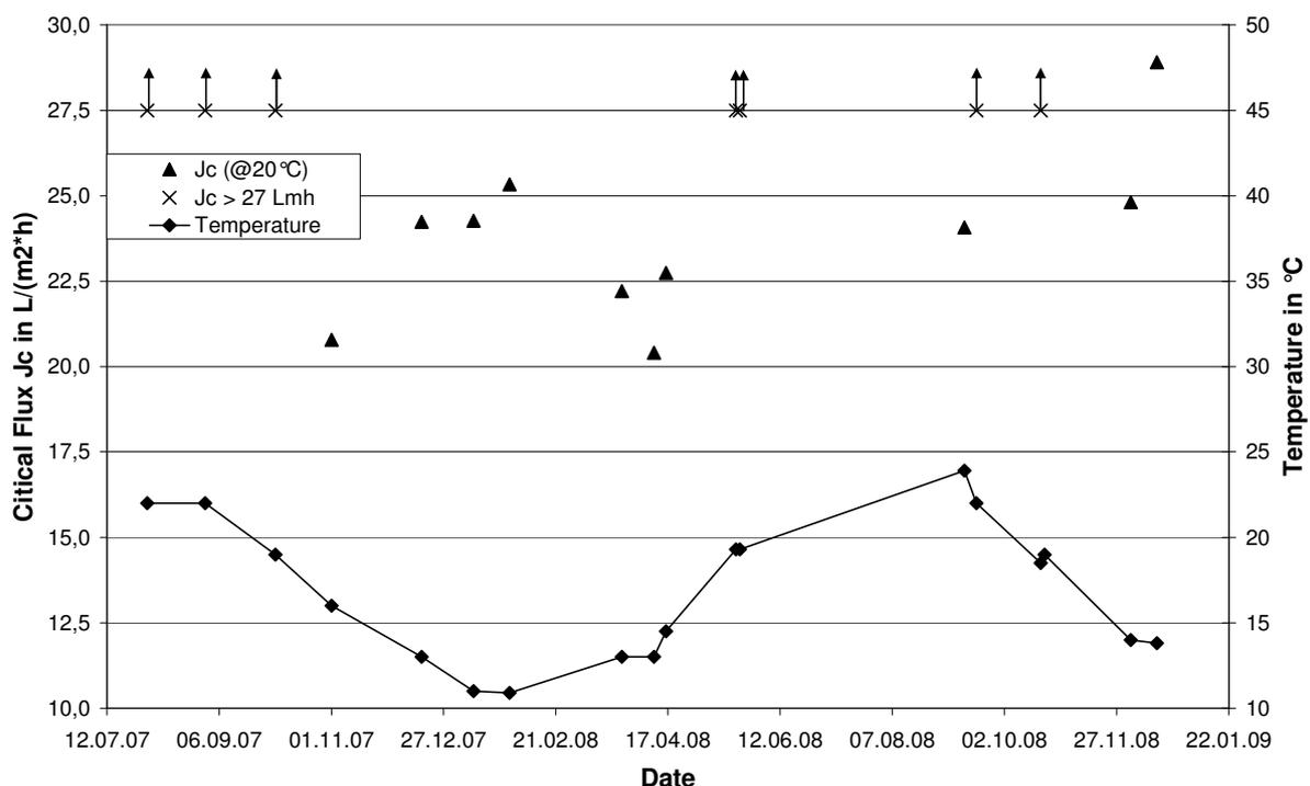
**Figure 46: Critical flux measurements (installed modules)**
