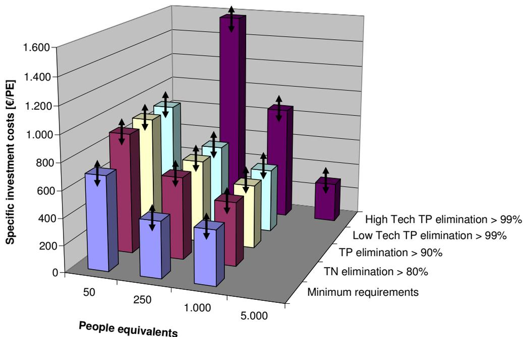
Figure 23: Investment costs according to plant size and effluent quality
