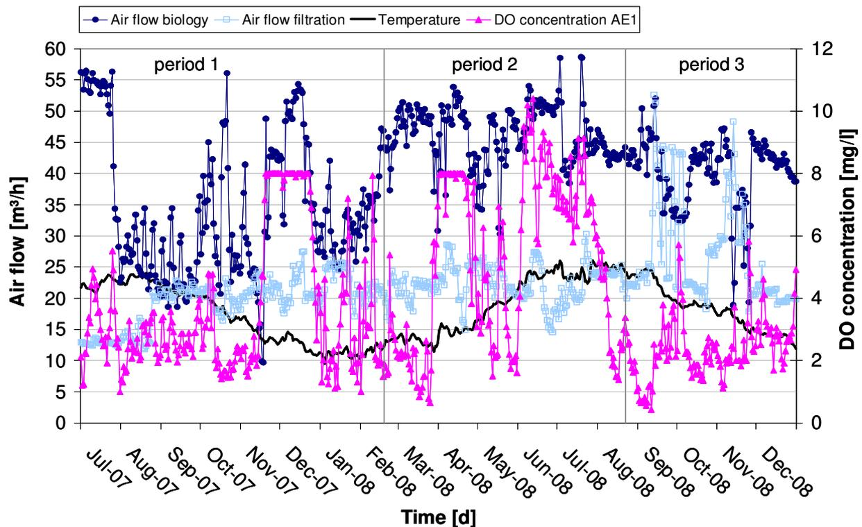
**Figure 15: Air flow of biology and filtration, sludge temperature and DO concentration over time (24h average)**
