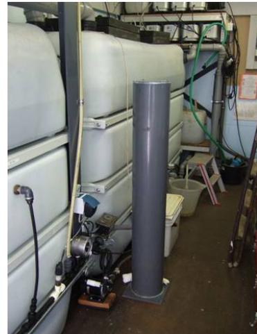
**Picture 3: Adsorption filter**
