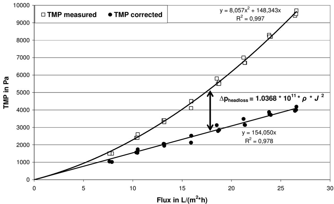
Figure 39: Head loss determination for module 1
