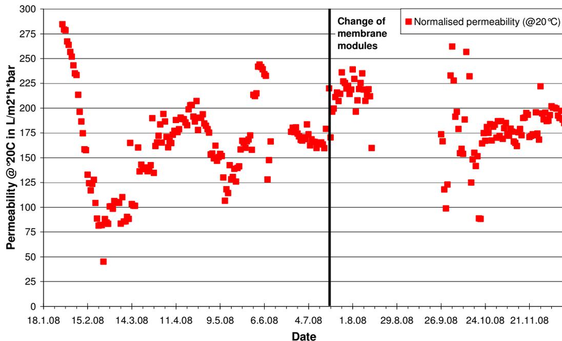
**Figure 66: Normalized permeability (@20 °C)**
