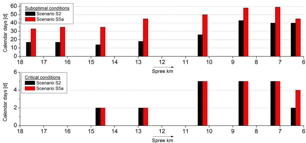
Figure 27: Simulated number of calendar days with suboptimal (upper panel) and critical DO conditions (lower panel) for i) the sewer status 2020 (S2) and ii) the sewer status 2020 with increased temperature (+1.9 K) (S5a). The arrow indicates the flow direction of the River Spree.
