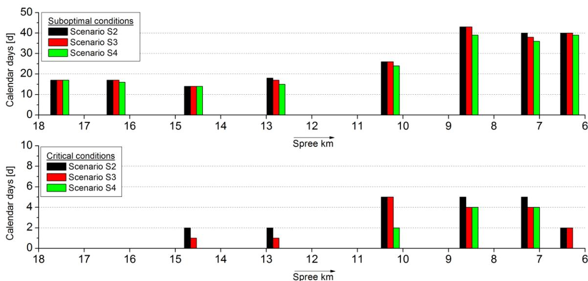
Figure 24: Simulated number of calendar days with suboptimal (upper panel) and critical DO conditions (lower panel) for i) the sewer status 2020 (S2), ii) the sewer status 2020 with increased storage volume (S3) and iii) the sewer status 2020 with reduced impervious connected area (S4). The arrow indicates the flow direction of the River Spree.
