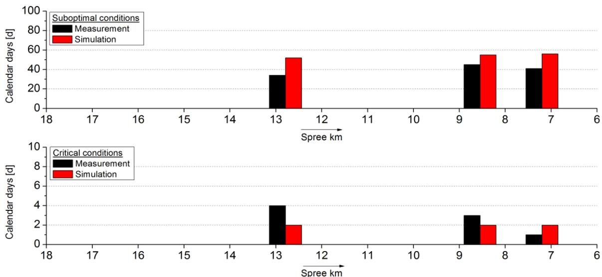
Figure 16: Number of calendar days with suboptimal (upper panel) and critical DO conditions (lower panel) according to measurements and simulations for the year 2010. The arrow indicates the flow direction of the River Spree.
