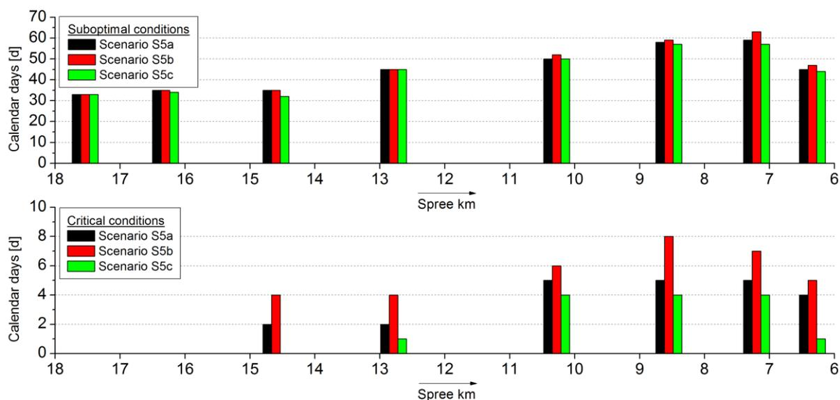
Figure 30: Simulated number of calendar days with suboptimal (upper panel) and critical DO conditions (lower panel) for i) the sewer status 2020 with increased temperature (+1.9 K) (S5a), ii) the sewer status 2020 with increased temperature (+1.9 K) and rain intensity (+20%) (S5b) and iii) the sewer status 2020 with increased temperature (+1.9 K) and reduced rain intensity (-20%) (S5c). The arrow indicates the flow direction of the River Spree.
