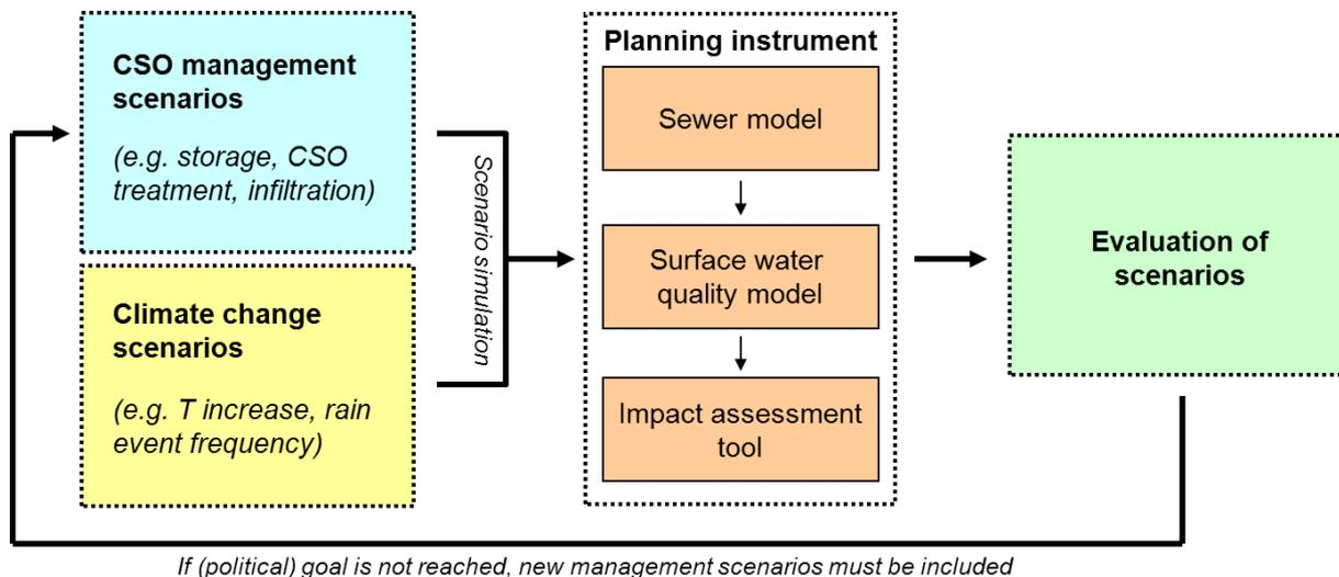
Figure 1: Schematic structure of the planning instrument and its application. External boundary conditions (such as global warming or changed water use) are yellow, CSO management scenarios are blue, the planning instrument is orange and the actual output of the instrument is green (adapted from Matzinger et al., 2012).
