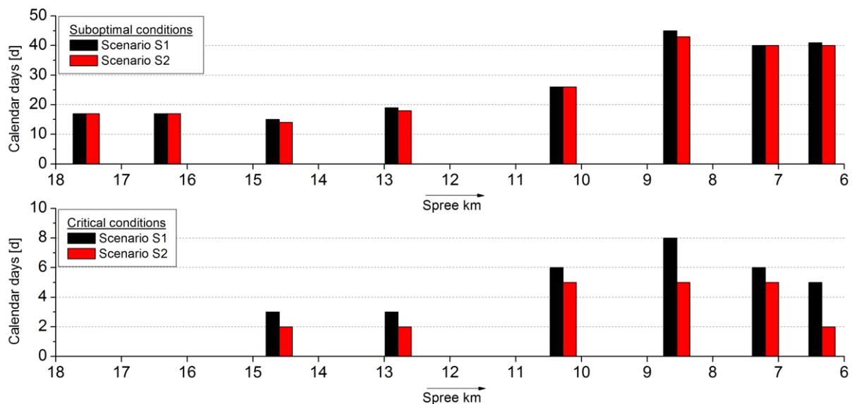
Figure 21: Simulated number of calendar days with suboptimal (upper panel) and critical DO conditions (lower panel) for i) the sewer status 2010 (S1) and ii) the sewer status 2020 with implemented sewer rehabilitation measures (S2). The arrow indicates the flow direction of the River Spree.
