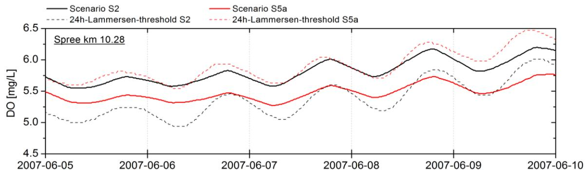
Figure 28: Simulated DO concentrations and 24h-Lammersen-thresholds for the sewer status 2020 (S2) and the sewer status 2020 with increased temperature (+1.9 K) (S5a) at Spree km 10.28.
