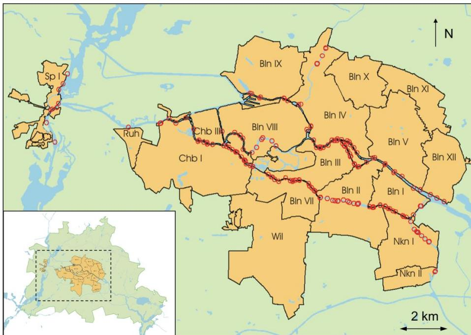
Figure 2: Map of the combined sewer system of Berlin with its subcatchments and CSO outlets (red circles) into the Berlin River Spree and its side channels
