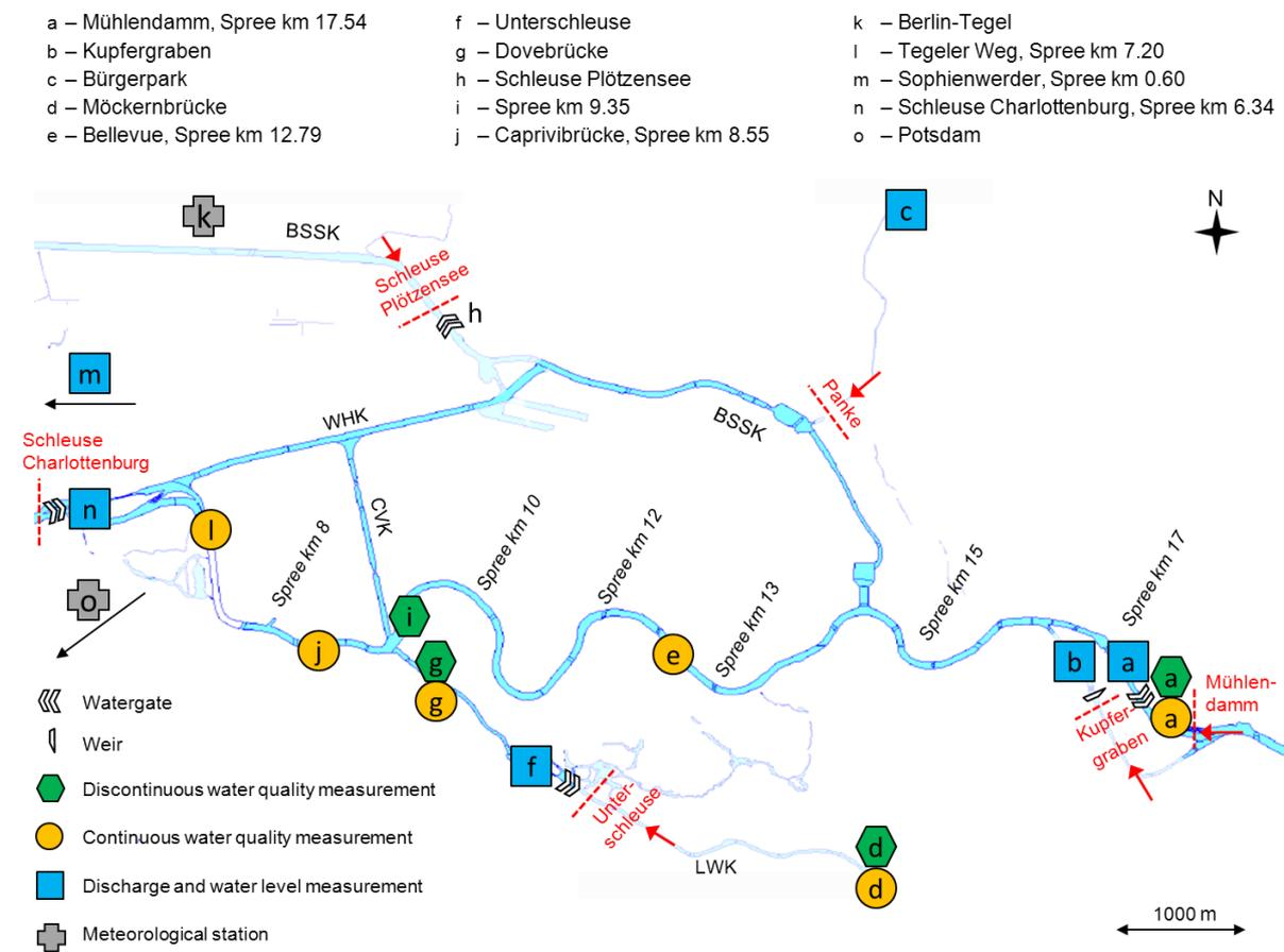
Figure 4: Map of modelled water system (blue), model boundaries (red) and measurement stations (green, yellow and blue symbols, adapted from SenStadt, 2004 and WSV, 2012). According to conventions of the Water Shipping Authority, the merging point of Havel and Spree in Berlin-Spandau is defined as Spree km 0. Abbreviations indicate BSSK: Berlin-Spandauer Schifffahrtskanal, CVK: Charlottenburger Verbindungskanal, LWK: Landwehrkanal and WHK: Westhafenkanal.
