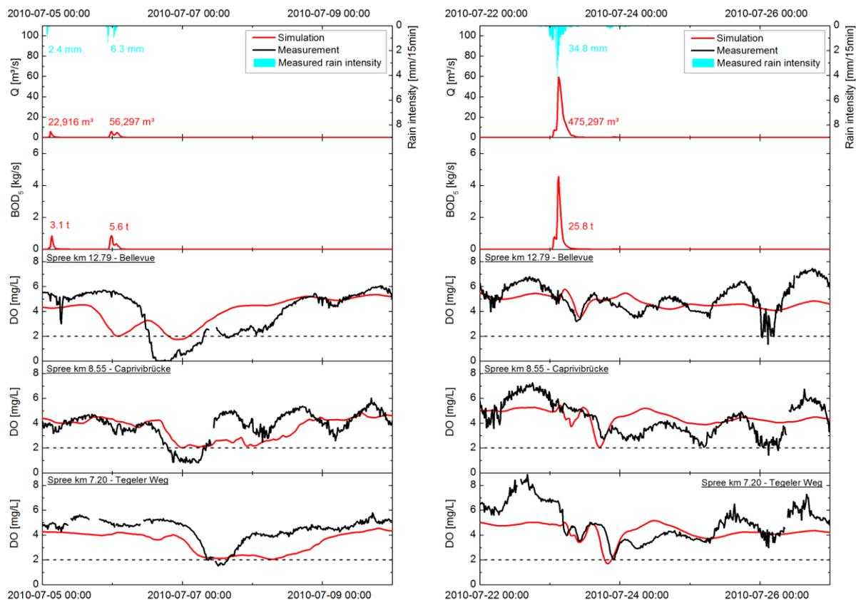
Figure 10: Simulated discharge and BOD<sub>5</sub> mass flow for all simulated CSO outlets and measured rain intensity within the investigation area as well as simulated and measured DO concentrations for two particular CSO events in July 2010 at Spree km 12.79 (Bellevue), Spree km 8.55 (Caprivibrücke) and Spree km 7.20 (Tegeler Weg). Dotted line marks the critical concentration for the asp (*Aspius aspius*).
