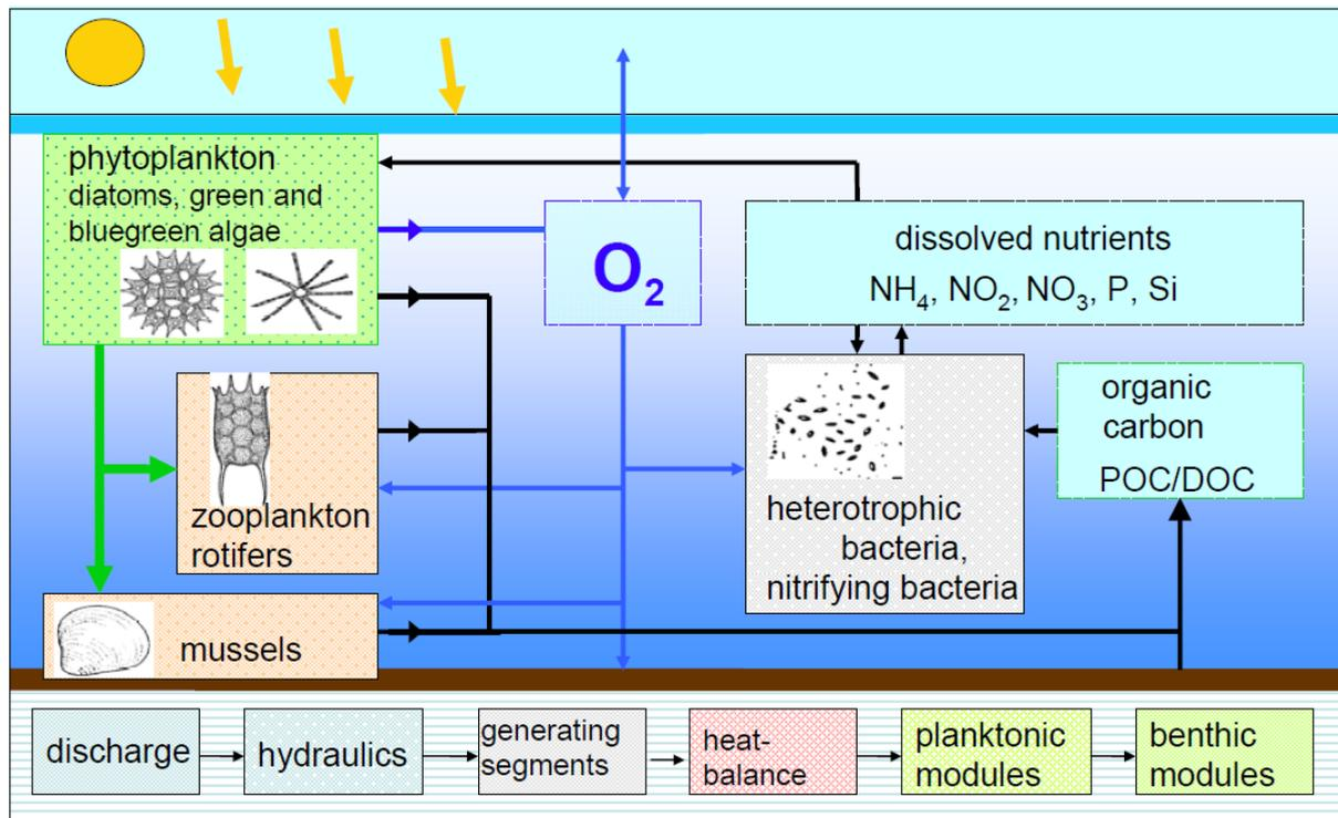
Figure 3: Modules and functionality of the river water quality model Hydrax/QSim (Kirchesch, 2004). POC=particulate organic carbon, DOC=dissolved organic carbon.
